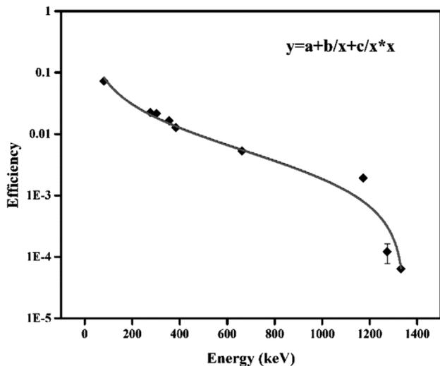
Fig. 1 — Efficiency calibration of CZT detector.
