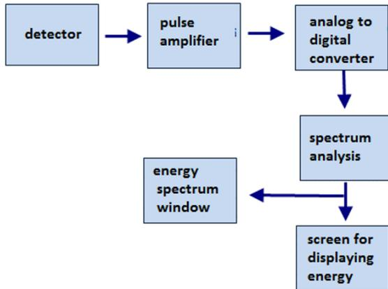
Fig. 2 — General view of the gamma ray spectrometer.
