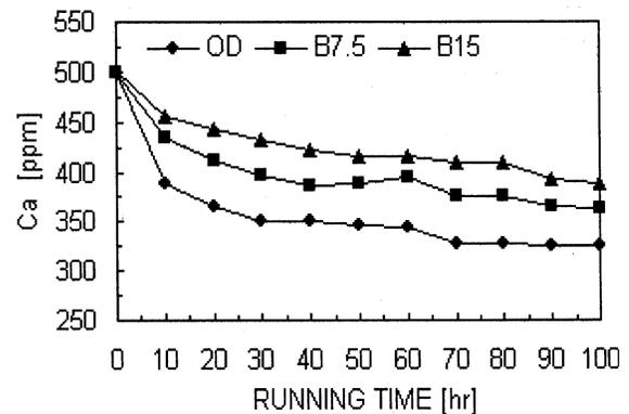
Fig. 11 — Ca concentration vs engine operation time
