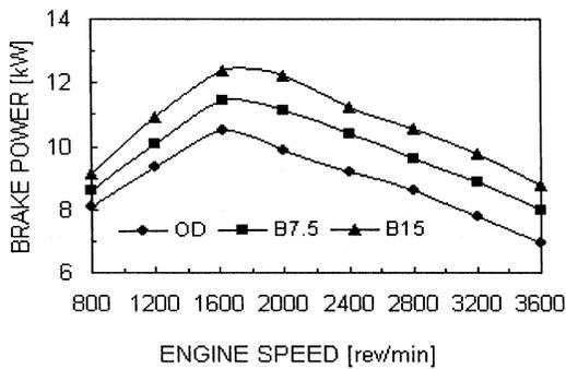
Fig. 2 — Brake power vs engine speed
