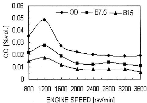
Fig. 4 — CO concentration vs engine speed
