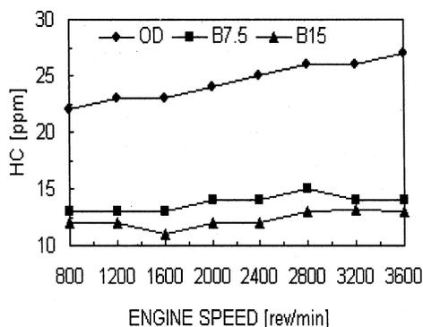
Fig. 5 — HC concentration vs engine speed
