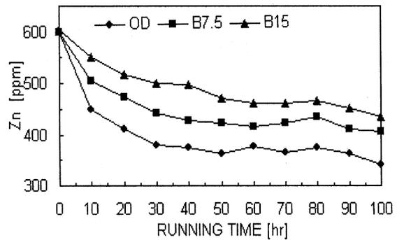
Fig. 10 — Zn concentration vs engine operation time
