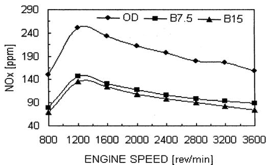
Fig. 3 — NOx concentration vs engine speed
