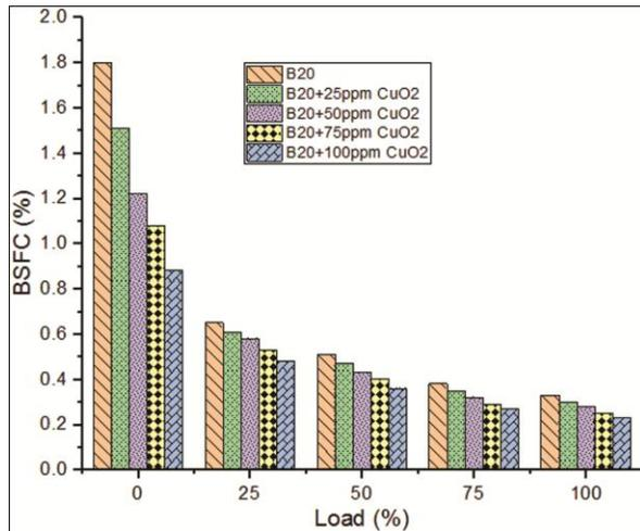
Figure 2 — Variation of Brake specific fuel consumption with load
