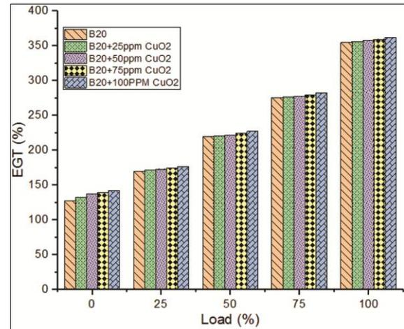
Figure 3 — Variation of Exhaust gas temperature with load
