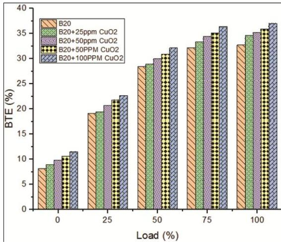
Figure 1 — Variation of Brake thermal efficiency with load
