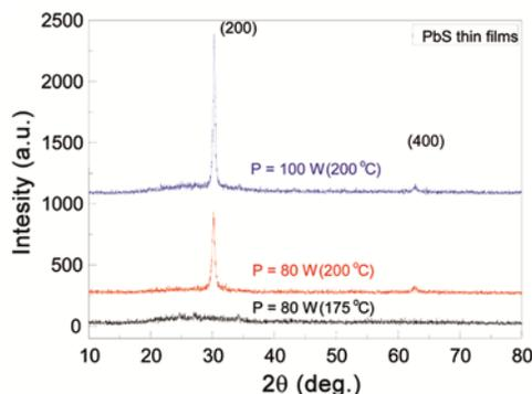
Fig. 1 – XRD-pattern of PbS thin films with respect to the variation of RF-power (P) and temperature (T), (a) P = 80 W, T =  $175^\circ\text{C}$ , (b) P = 80 W, T =  $200^\circ\text{C}$  and (c) P = 100 W, T =  $200^\circ\text{C}$ .
