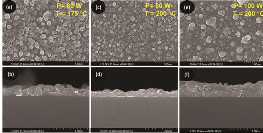
Fig. 3 – FE-SEM microscopic images of PbS thin films, (a) and (b) surface and cross-section at P = 80 W, T = 175 °C, (c) and (d) surface and cross-section at P = 80 W, T = 200 °C, (e) and (f) surface and cross-section at P = 100 W, T = 200 °C.
