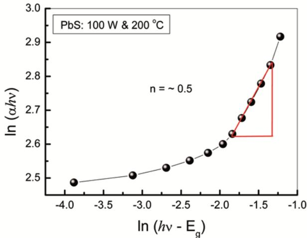
Fig. 6 – Plot of  $\ln(\alpha h\nu)$  versus  $\ln(h\nu - E_g)$  of as-grown sputtered PbS thin film (power = 100 W and growth temperature = 200 °C). The slope ( $n$ )  $\sim 0.5$  shows the direct type transition.
