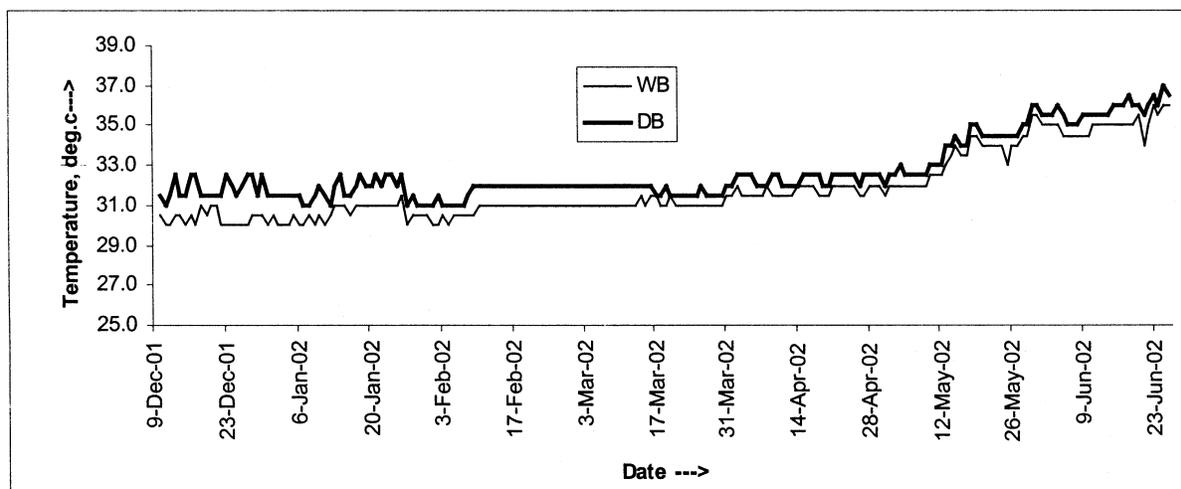
Fig. 3 — Temperature variation (Goaf return) of BG-2A, Block-C Panel
