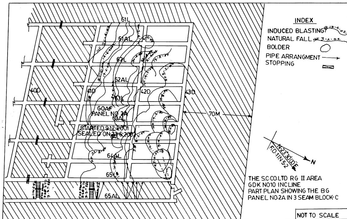
Fig. 1 — Blasting gallery panel 2A of Block -C of GDK-10, Incline mine
