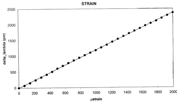
Fig. 8—Shift of Bragg wavelength with strain
