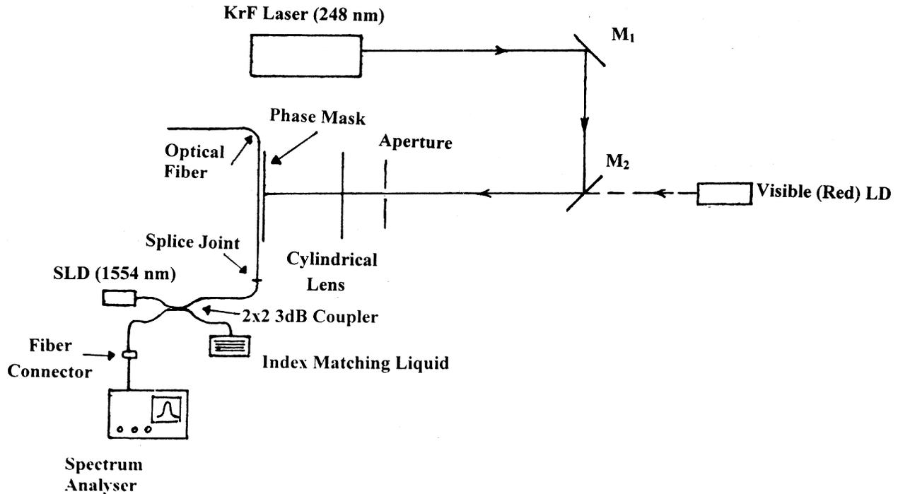
Fig. 3—Schematic of the set up used for writing FBGs
