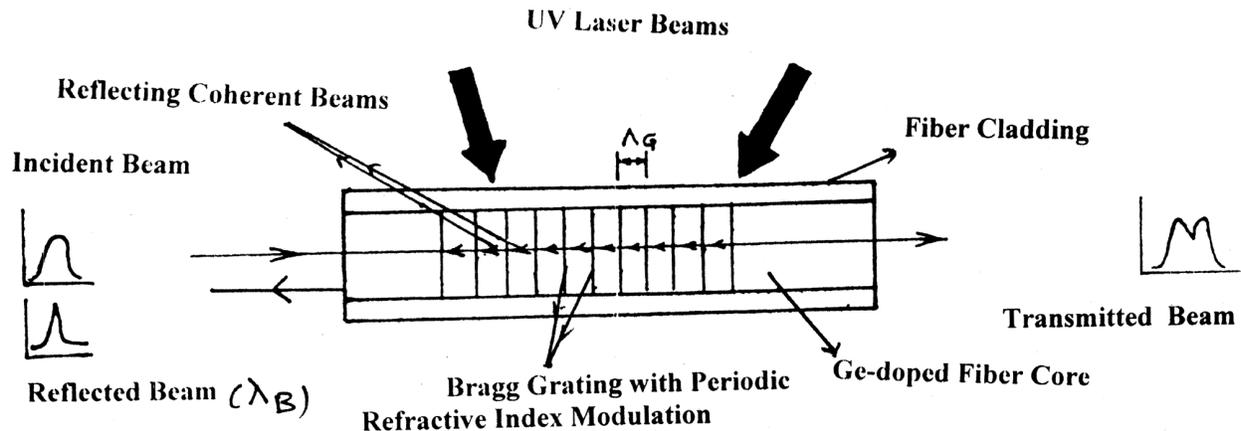
Fig. 1—Schematic diagram of an in-fibre Bragg grating
