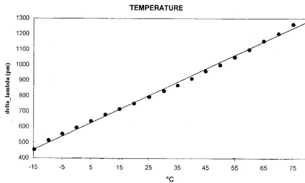
Fig. 9—Shift of Bragg wavelength with temperature
