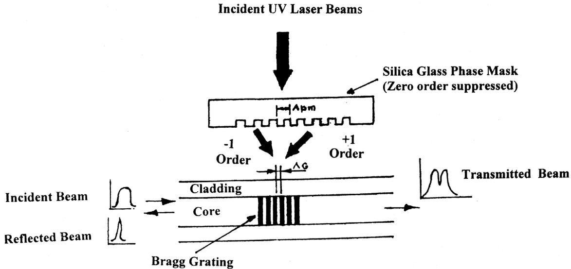
Fig. 2—Schematic representation of a typical set up for inscribing Bragg gratings in optical fibers
