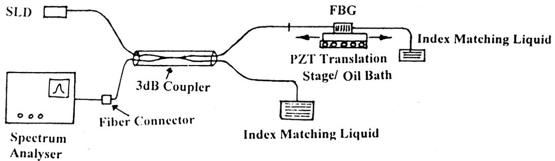
Fig. 7—Schematic of the experimental set up used for characterisation of FBGs.
