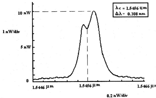
Fig. 10—Reflection spectrum of a FBG inscribed on both sides of a fiber splice
