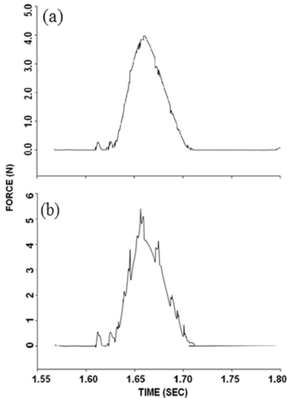
Fig. 2 — Force distribution on Slot pin (a) and Force distribution on lead screw (b)
