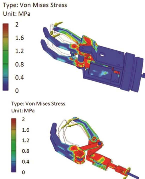
Fig. 3 — Von Mises stress distribution in Arm prosthesis and lead screw assembly
