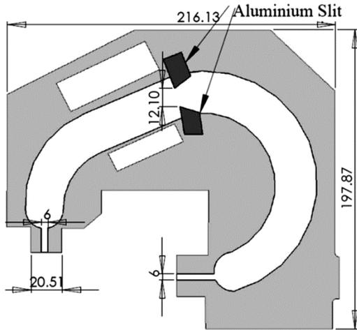
Fig. 6 – Cross sectional view of vacuum chamber with aluminium slit.
