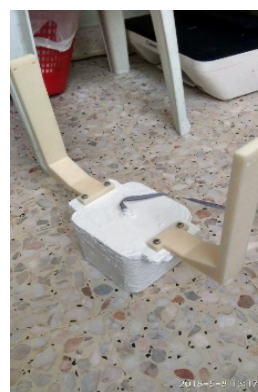
Fig. 6 — Pixy sensor pressure housing with supportive arms
