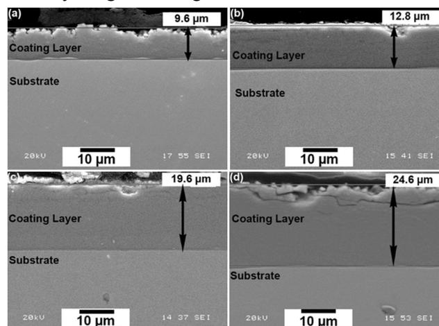
Fig. 1 — SEM Micrographs of aluminized Inconel 718 alloy at 600°C (a) 2h, (b) 4h and 650°C (c) 2h, (d) 4h
