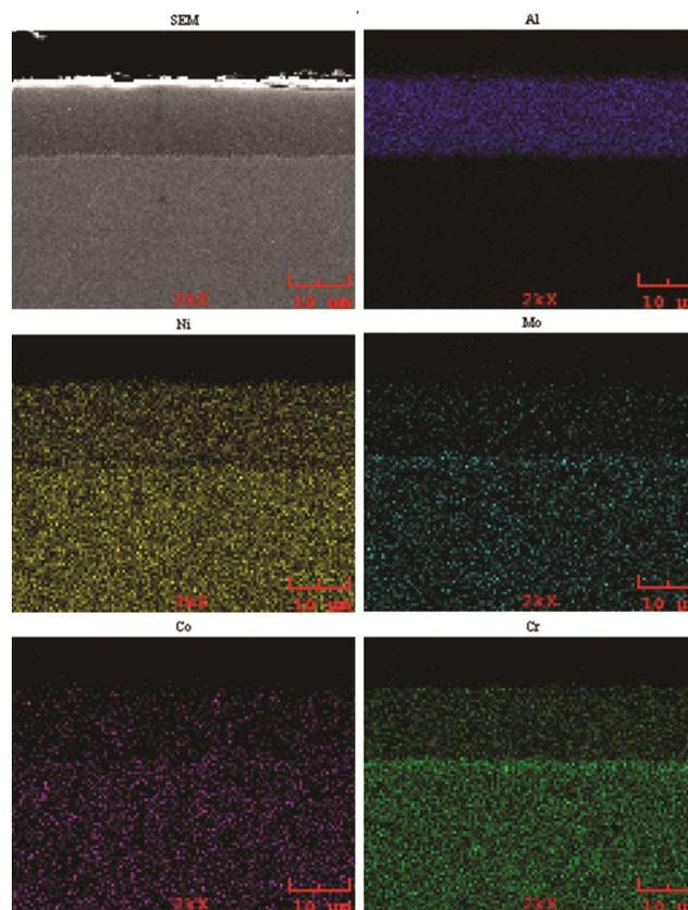
Fig. 2 — SEM-MAP analysis of Inconel 718 alloy pack aluminized at 600°C for 4 h
