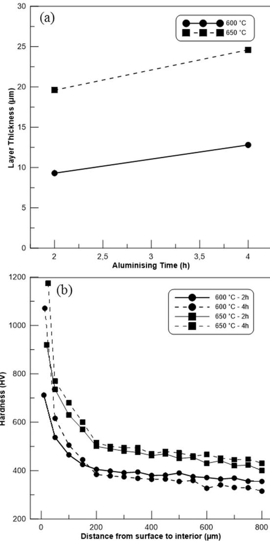
Fig. 4 — Variation of (a) aluminising layer thickness versus aluminising time, (b) hardness versus distance from surface to interior for pack aluminised Inconel 718 alloy
