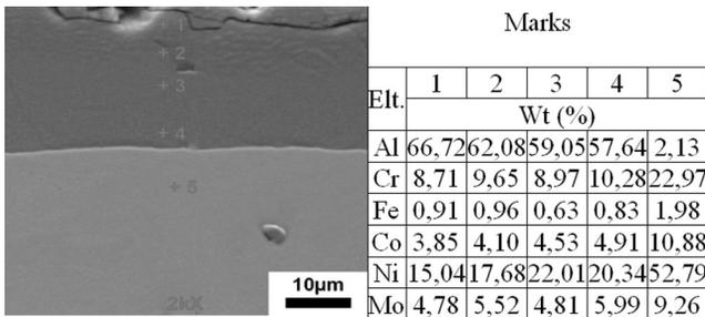
Fig. 3 — SEM-EDS analysis of Inconel alloy pack aluminized at 650°C for 4 h.
