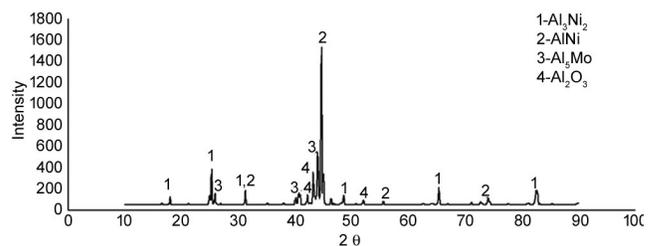
Fig. 5 — XRD analysis of Inconel 718 alloy pack aluminized at 650°C for 4 h.
