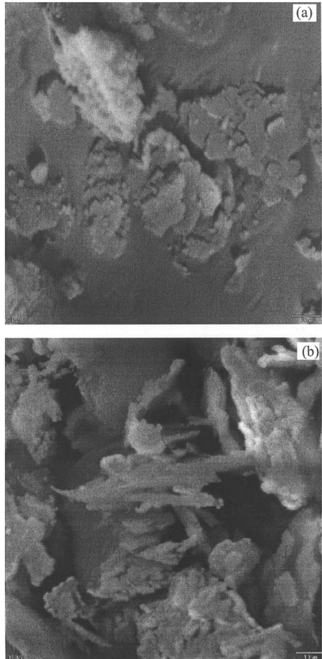
Fig. 2— (a) The photograph of the original clay under the scanning electron microscope (magnification 10000), (b) The photograph of the clay contaminated with the leachate (magnification 10000)
