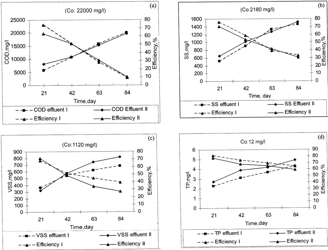
Fig. 3—Concentrations of a) COD, b) SS, c) VSS and d) TP
