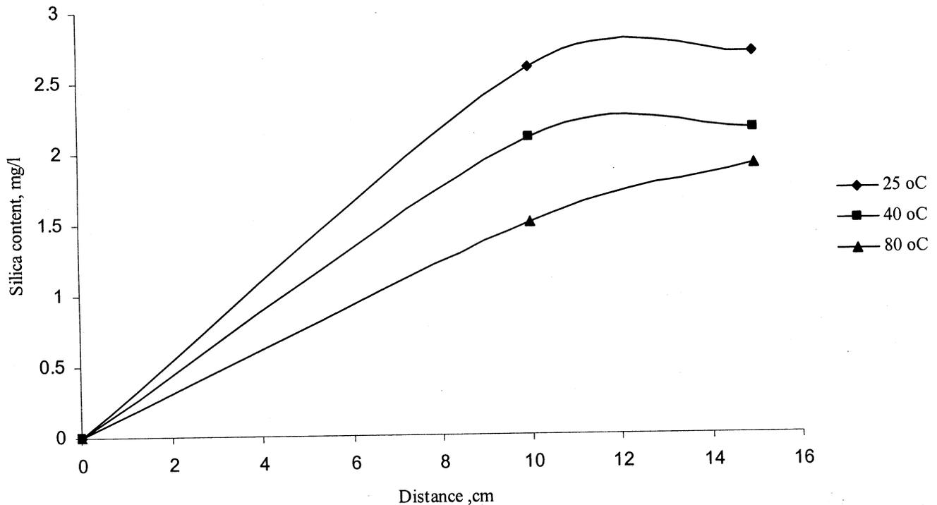
Fig.1— Distance vs silica content in sedimentation (time-30min, flocculant dose-3%)
