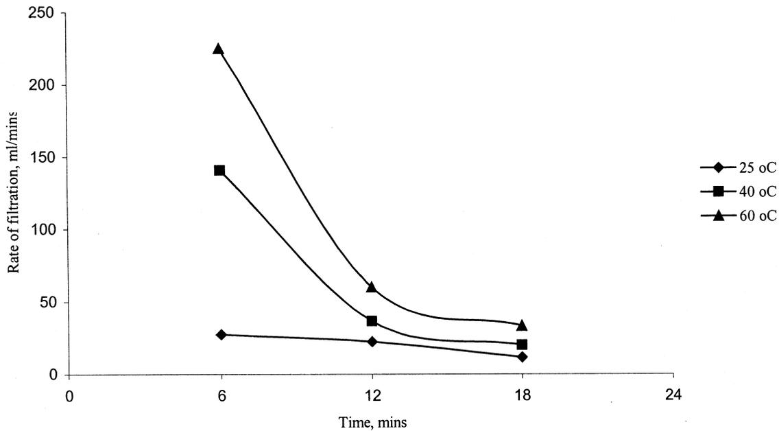
Fig 4— Rate of filtration vs time at different temperature
