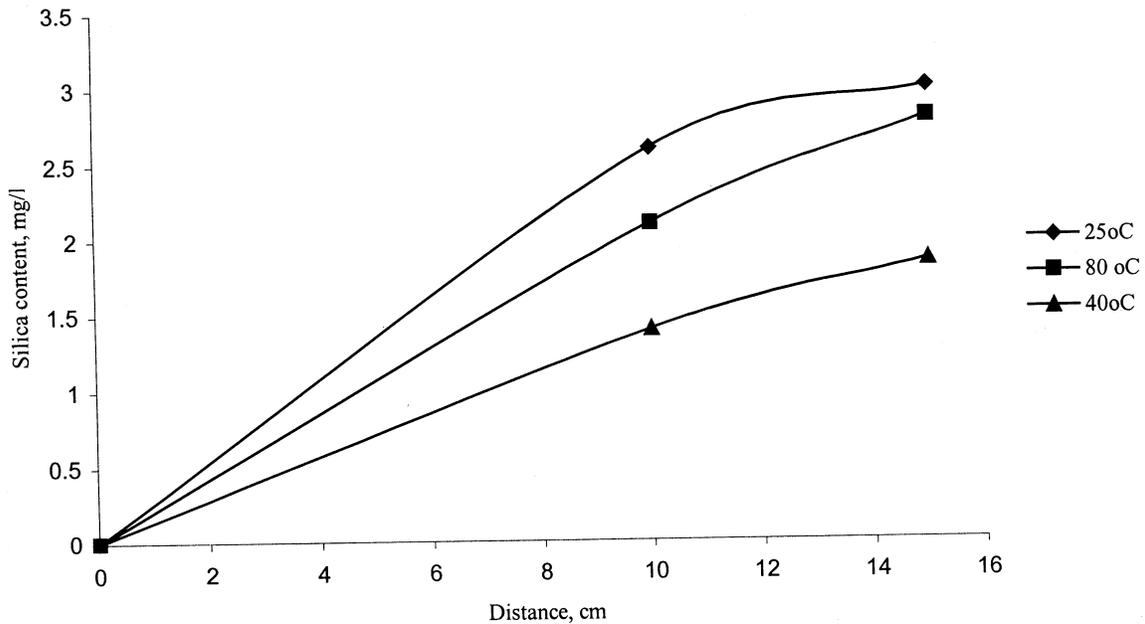
Fig. 2— Distance vs silica content in sedimentation (time=60min, flocculant dose=3%)
