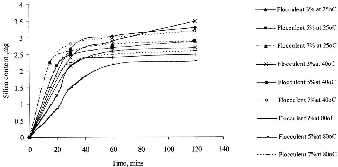
Fig 3— Silica content vs time at different temperature and flocculent dosage (distance=15 cm)
