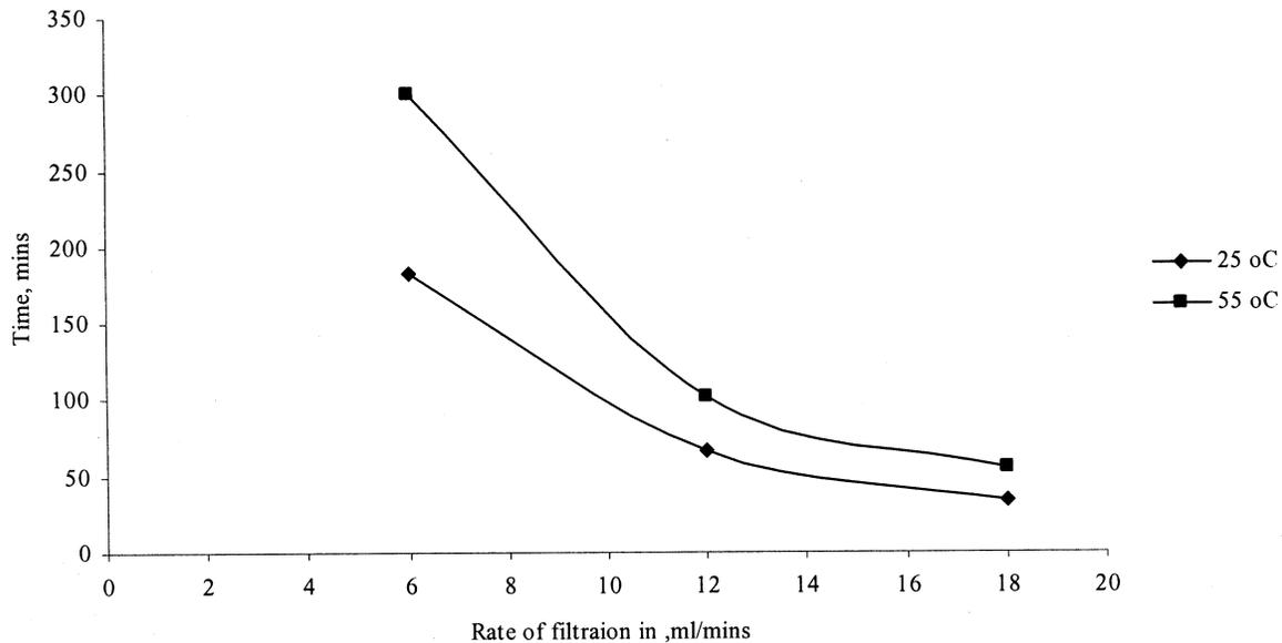
Fig. 5— Rate of filtration vs time at different temperature using flocculent
