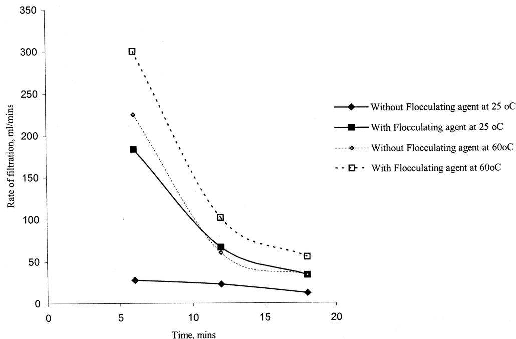
Fig. 6— Rate of filtration vs time at room temperature
