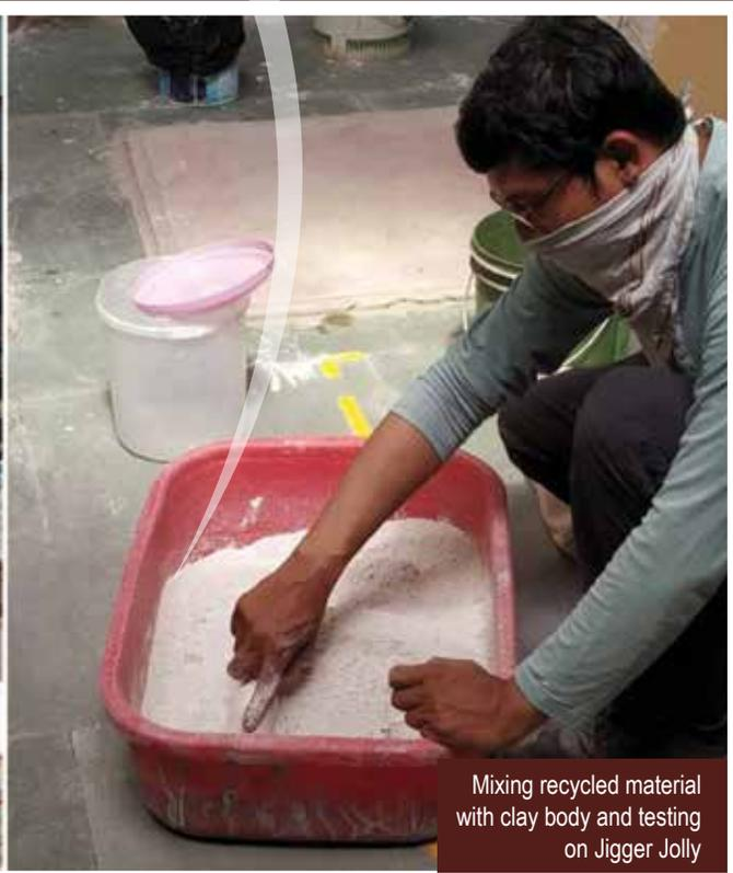
Mixing recycled material with clay body and testing on Jigger Jolly
