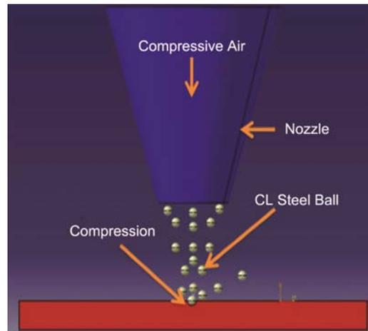
Fig. 1 — Schematic representation of shot peening process
