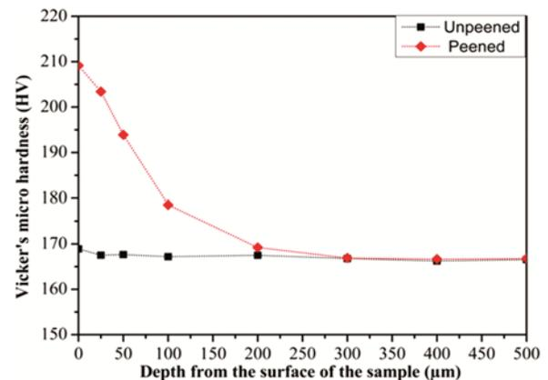
Fig. 5 — Hardness chart measured across the surface
