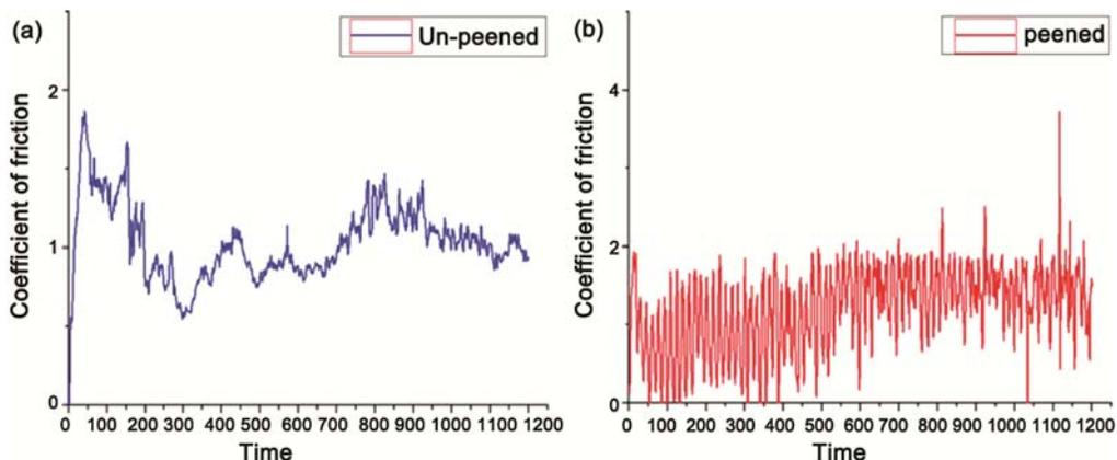
Fig. 10 — Coefficient of friction of (a) un-peened surface and (b) peened surface
