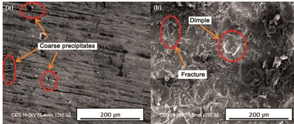
Fig. 3 — SEM image of (a) un-peened and (b) peened surface
