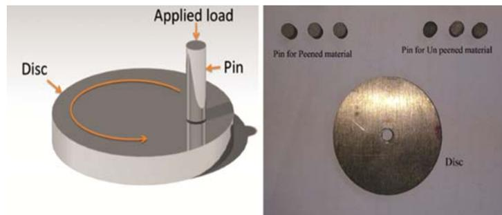
Fig. 2 — Specimens used for friction and wear measurement
