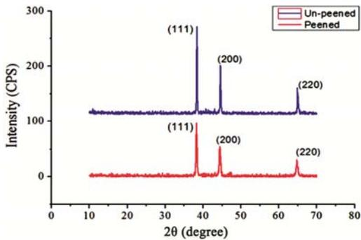
Fig. 6 — XRD of (a) peened and (b) un-peened
