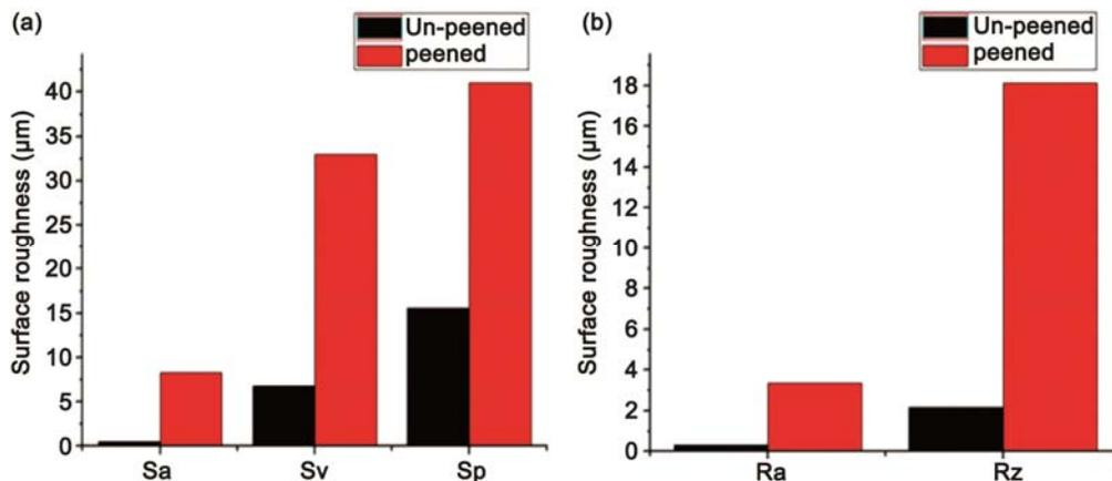
Fig. 9 — 3D Surface parameters of (a) un-peened and (b) peened aluminium 7075-T651 alloy
