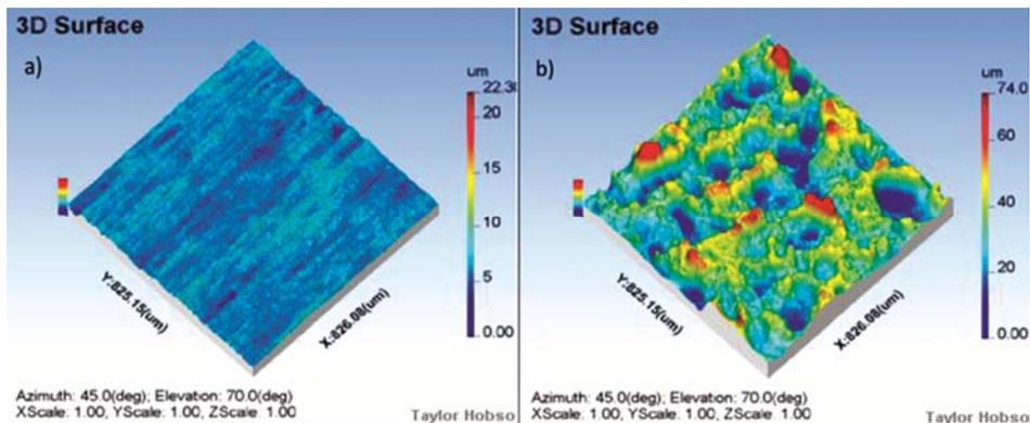
Fig. 8 — 3D Topographies of (a) un-peened and (b) Peened aluminium 7075-T651 alloy
