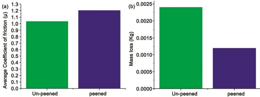
Fig. 11 — Images of (a) average coefficient of friction and (b) mass loss
