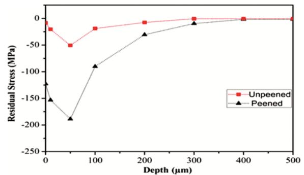
Fig. 7 — Depth-wise compressive residual stresses profile for the un-peened and peened aluminium 7075-T651 alloy
