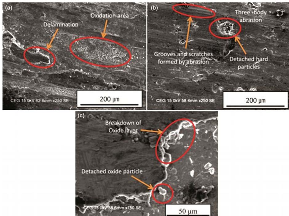
Fig. 12 — SEM image of wear track of (a) un-peened and (b & c) peened aluminium 7075-T651 alloy
