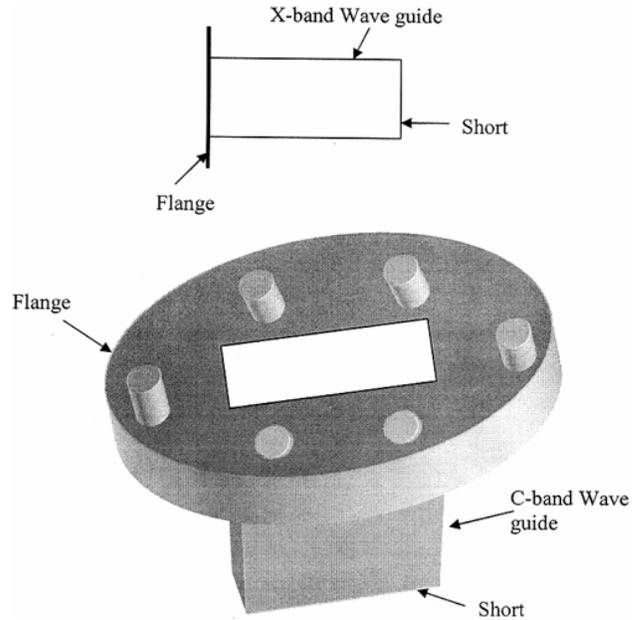
Fig. 3—Construction of the sample holder for X-band and C-band microwave bench
