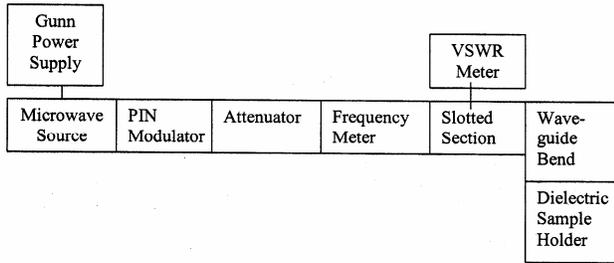
Fig. 2—The experimental set up for the two-point method at X-band microwave frequency
