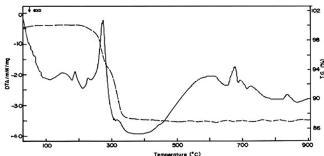
Fig. 6 — TGA-DTA curves of coumarine doped GLS crystal.
