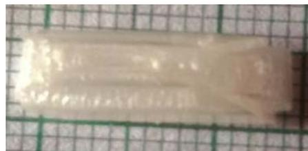
Fig. 1 — Photograph of coumarine doped GLS crystal.
