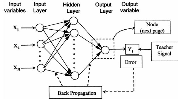
Fig. 2—Typical structure of artificial neural network.
