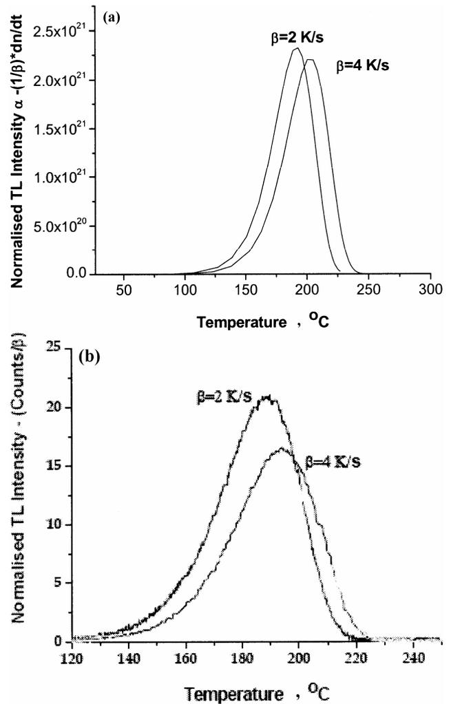
Fig. 3 — Normalized TL glow curves: (a)  $(\text{TL}/\beta)$  corresponding to Fig. 1b, (b) (experimental- $\text{TL}/\beta$ ) corresponding to Fig. 2b.
