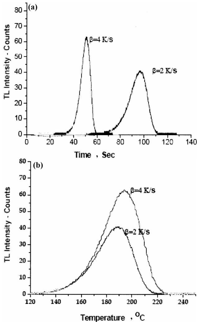
Fig. 2 — TL glow curves (experimental) for  $\alpha$ - $\text{Al}_2\text{O}_3\text{:C}$  at two different heating rates plotted in: (a) time, (b) temperature. The dose (beta) given to the sample was 5 mGy
