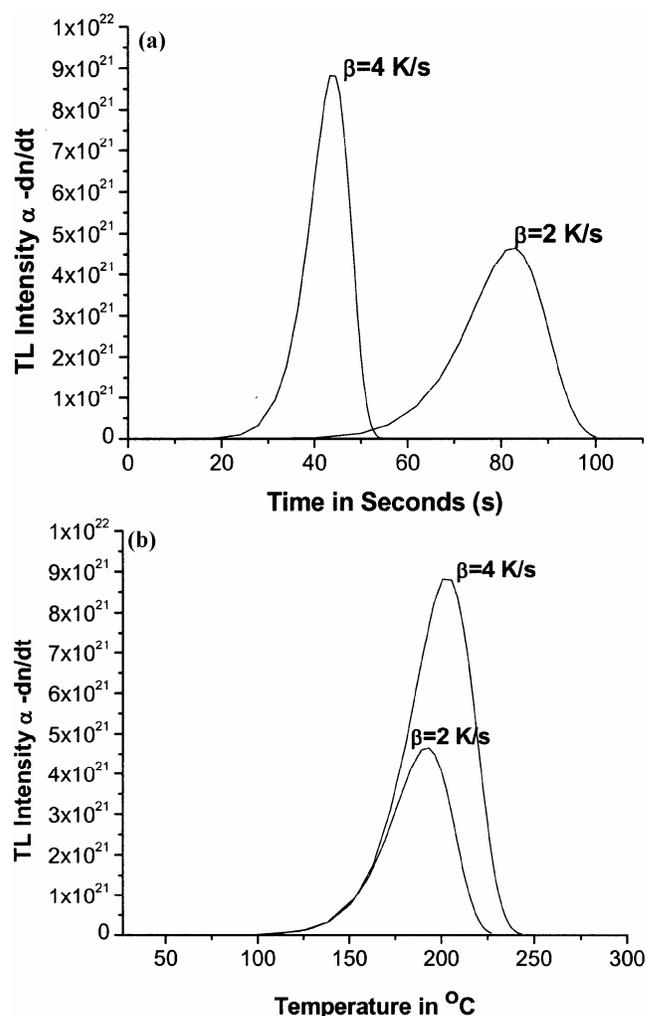
Fig. 1 — Plot of TL intensity (theoretical) with respect to: (a) time, (b) temperature. The parameters assumed are, activation energy,  $E = 1.1\text{ eV}$ , frequency factor,  $s = 10^{11}\text{ Hz}$ ,  $T_0 = 300\text{ K}$  and number of trapped electrons,  $n_0 = 10^{23}\text{ m}^{-3}$
