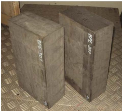
Fig. 1 — BPE (30%) slab used in experiment.
