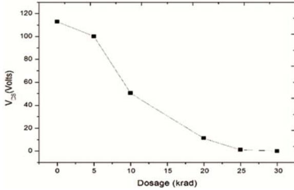
Fig. 2 — Plot of  $V_{DS}$  as a function of gamma dose for MOSFET 2N6796.
