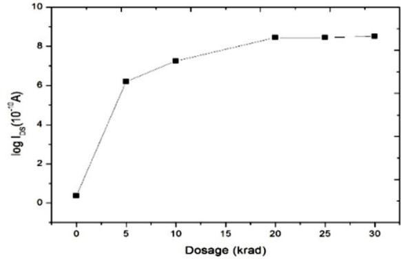
Fig. 4 — The drain to source leakage current as a function of gamma dose in MOSFET 2N6796.
