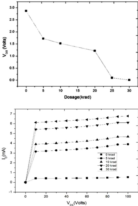
Fig. 3(a) — Gate threshold voltage ( $V_{GS}$ ) as a function of gamma dose for MOSFET 2N6796 and (b) sub threshold output characteristics of MOSFET 2N6796.
