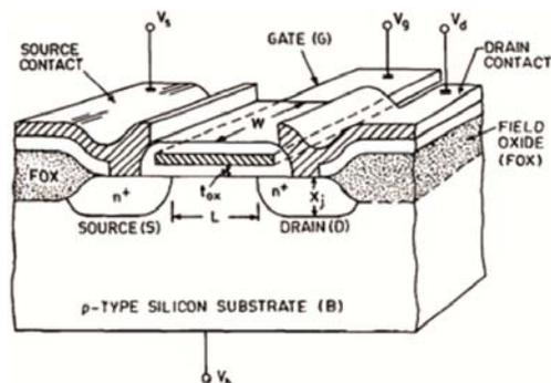
Fig. 1 — Schematic diagram of MOSFET.
