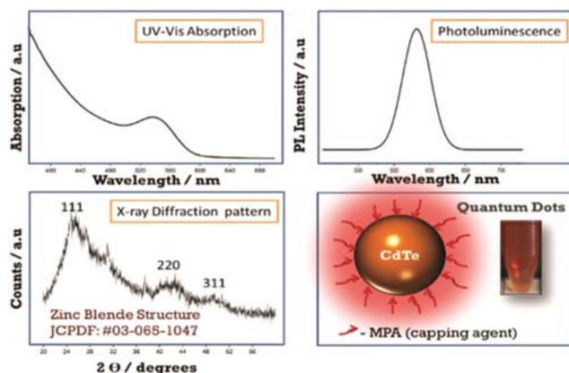
Fig. 2 — UVS spectra and PLS spectra (first row). XRD spectra and vial capture of CdTe QDs (second row).
