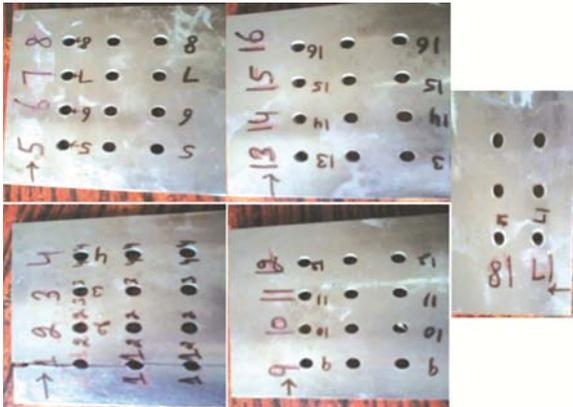
Fig. 2 – Drilled holes on D2 steel with abrasive assisted drilling
