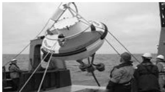
Fig 2- The deployment of a DART™ buoy detection buoy (DART™).
