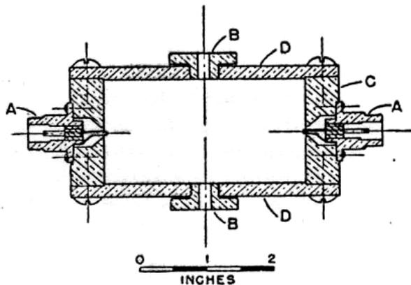
Fig. 1 — Cross-sectional view of cylindrical cavity resonator<sup>7</sup> (A — type N cable connectors, B — plugs to permit specimen to be inserted along axis of resonator, C — cylinder wall, and D — end plates perpendicular to cylinder axis)
