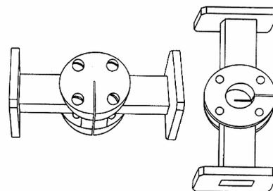
Fig. 2 — Cavity resonator for use with a single fibre at 26 GHz (ref. 27)
