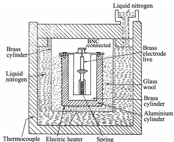
Fig. 3 — Test cell used for studying dielectric anisotropy<sup>9</sup>
