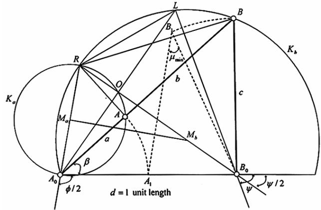
Fig. 3—Graphical solution of crank-rocker mechanism for  $\phi$
