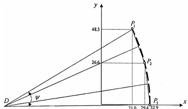
Fig. 2—Oscillation angle required for beat-up mechanism
