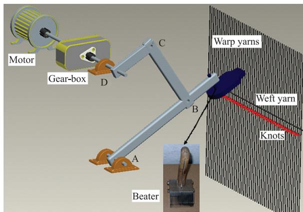
Fig. 1—Crank-rocker type beat-up mechanism placed in front of the handmade carpet loom
