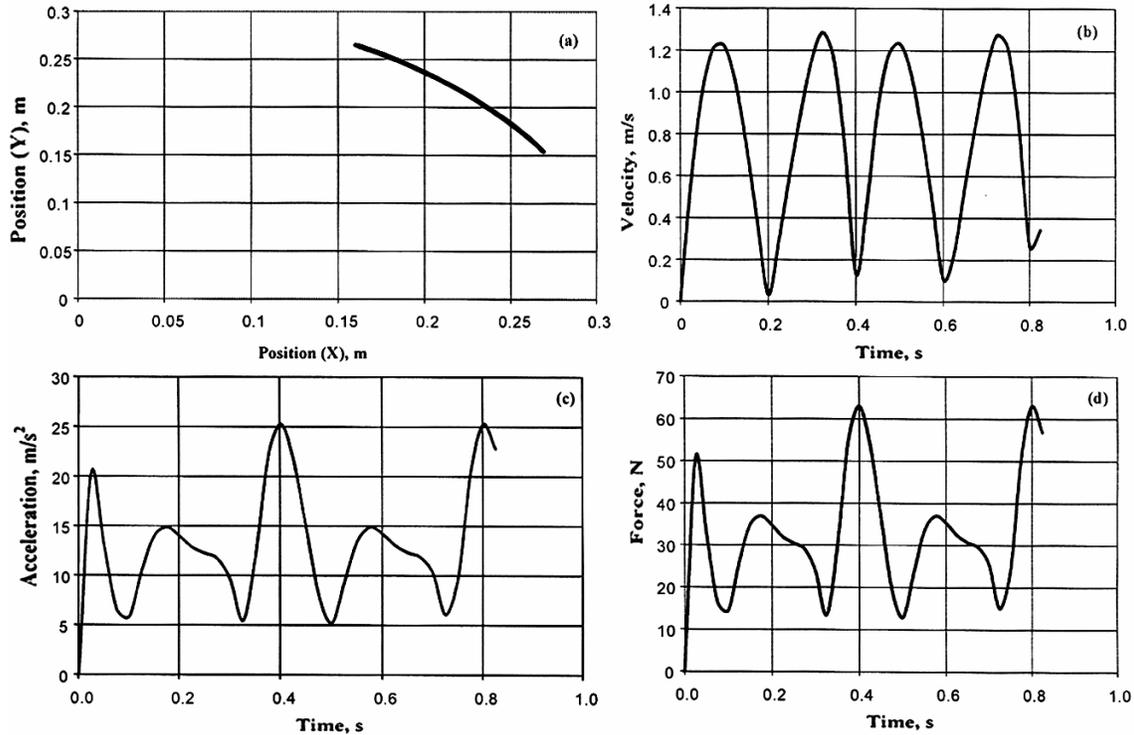
Fig. 6—Kinematics and dynamic analysis of the beater
