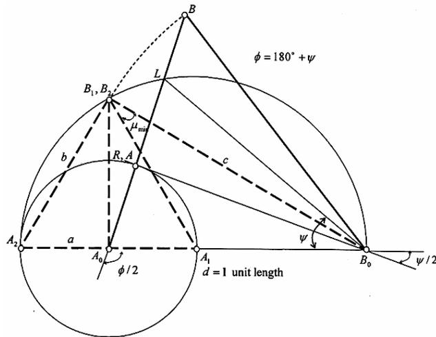
Fig. 4—Graphical solution of crank-rocker mechanism for  $\phi = 180^\circ + \psi$
