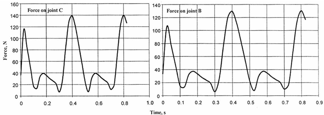
Fig. 7—Loads on pin joints C and B
