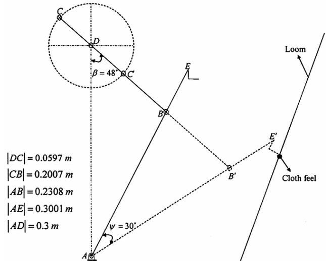
Fig. 5—Dimensions of links and motion of beat-up mechanism
