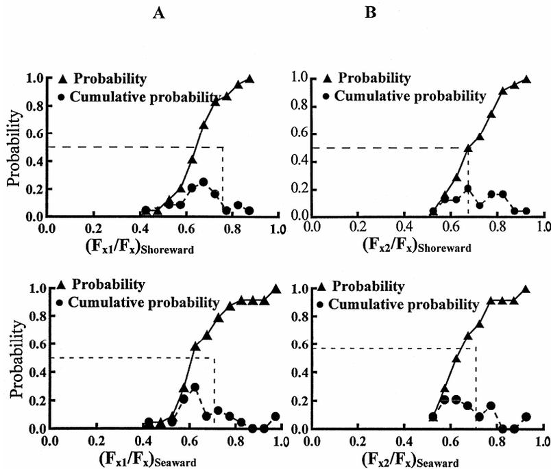
Fig. 7—Probability and Cumulative probability of force ratio of (A) vertical barrier and (B) inclined barrier.
