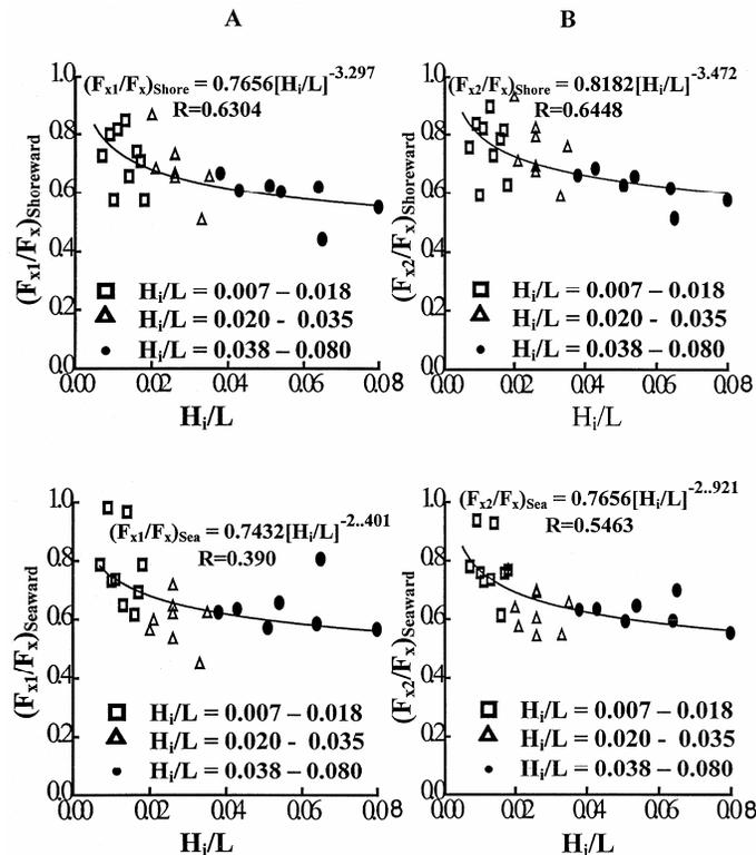
Fig. 4—Effect of  $H_i/L$  on wave force ratio for (A) vertical barrier and (B) inclined barrier.
