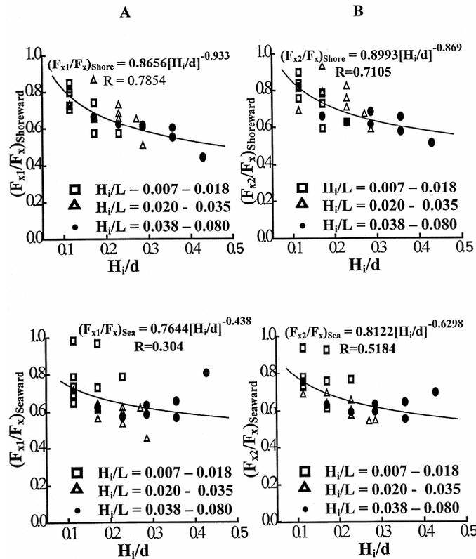
Fig. 3—Effect of  $H_i/d$  on wave force ratio for (A) vertical barrier and (B) inclined barrier.
