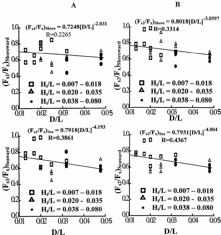
Fig. 5—Effect of  $D/L$  on wave force ratio for (A) vertical barrier and (B) inclined barrier.
