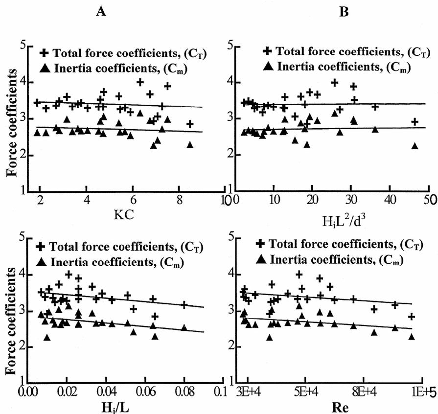
Fig. 2—Effect of Keulegan-Carpenter number, Ursell parameter, incident wave steepness and Reynolds number on the force coefficients on a vertical cylinder without perforated barrier
