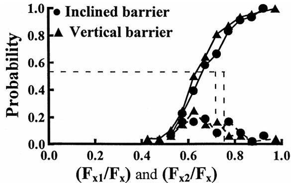
Fig. 8—Combined probability and cumulative probability of shoreward and seaward force ratio for (▲) vertical barrier and (●) inclined barrier.
