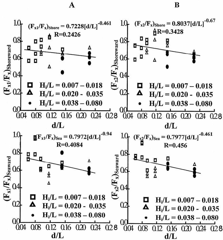
Fig. 6—Effect of  $d/L$  on wave force ratio for (A) vertical barrier and (B) inclined barrier.
