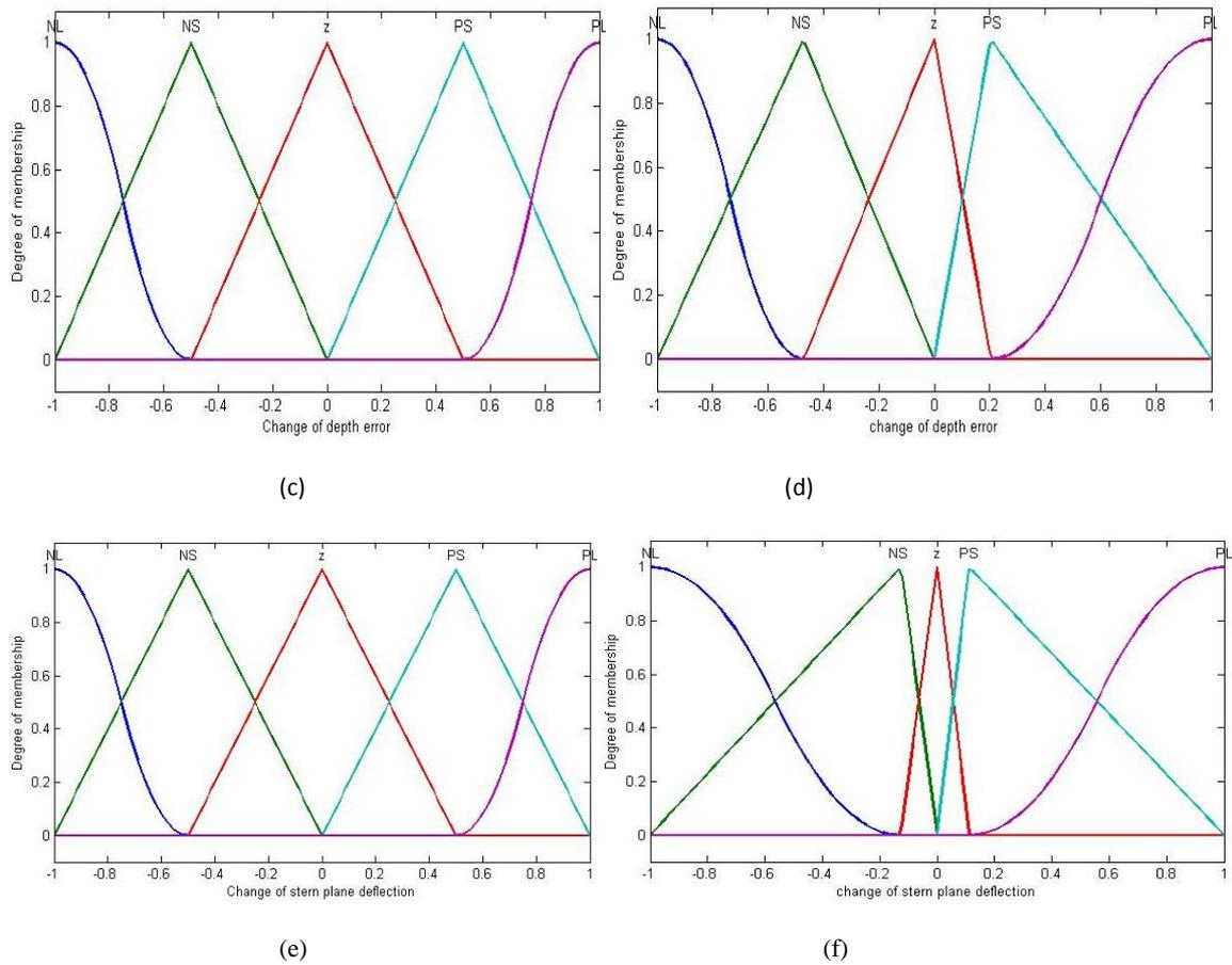
Fig.6 Membership functions for FLC (Before optimization) and GA-FLC (after optimization) (a,b) for depth error; (c,d) for depth error change; (e,f) for change in stern plane deflection
