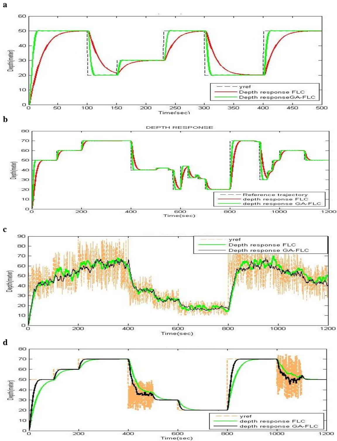
Fig.9 Trajectory tracking of DSRV through FLC and GA-FLC (a)  $y_{d1}$ -Reference trajectory-1 (b)  $y_{d2}$ - Reference trajectory -2 (c)  $y_{d3}$ -Wave disturbance added trajectory- 3 (full period of movement) (d)  $y_{d4}$ -Intermittently added wave disturbance trajectory- 4 (Wave disturbance introduced from 400 sec to 500sec and 1000sec to1100sec)
