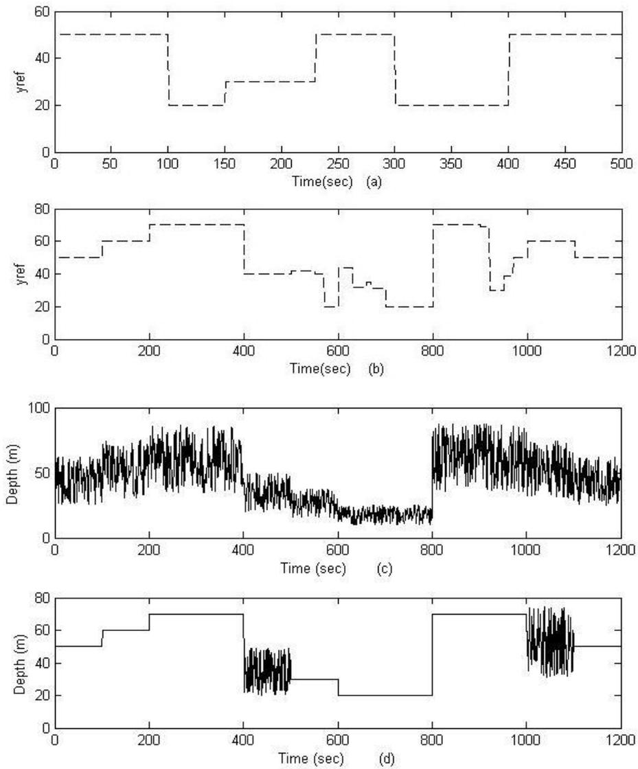
Fig. 5 Reference trajectories used in simulation (a)  $y_{d1}$  -Reference trajectory-1 (b)  $y_{d2}$ - Reference trajectory -2 (c)  $y_{d3}$ - Wave disturbance added trajectory- 3 (full period of movement) (d)  $y_{d4}$ .Intermittently added wave disturbance trajectory- 4
