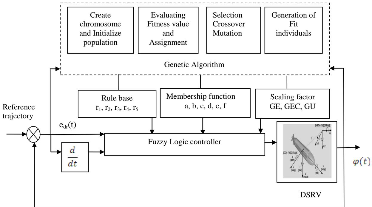
Fig. 2- GA based Fuzzy Logic Controller for DSRV
