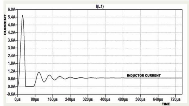
Fig. 14 Inductor current ripple of Boost Converter
