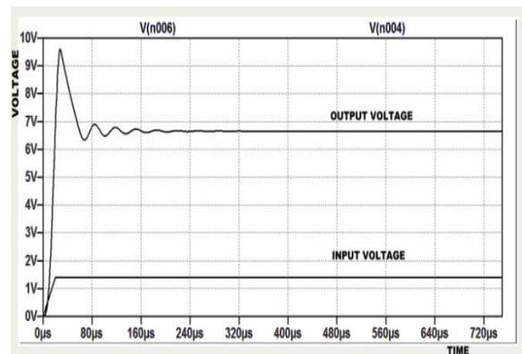
Fig. 10- Input and Output voltage of IBC
