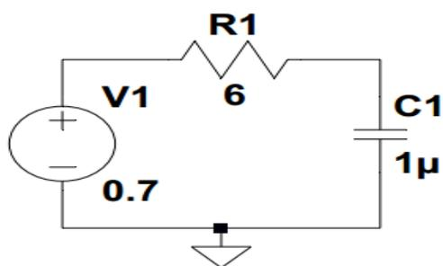
Fig. 1- Equivalent circuit of MFC
