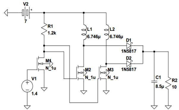
Fig. 5- Interleaved Boost Converter
