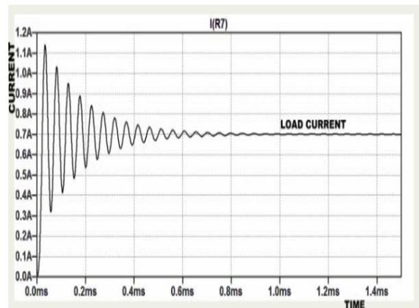
Fig. 18- Output current ripple of IBC using LTC3872
