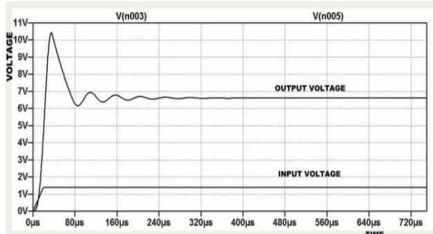
Fig. 13- Input and Output voltage of Boost Converter
