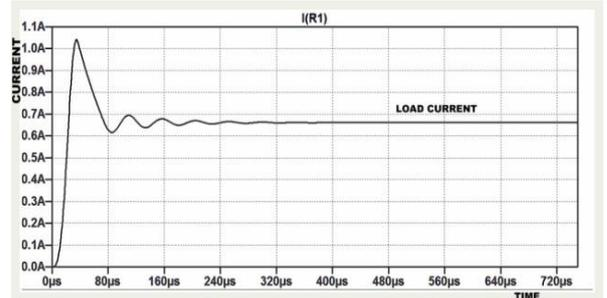
Fig. 15- Output current ripple of Boost Converter
