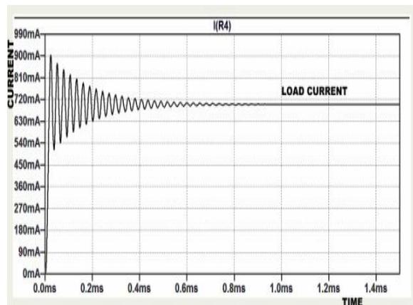
Fig. 21- Output current ripple of Boost Converter using LTC3872
