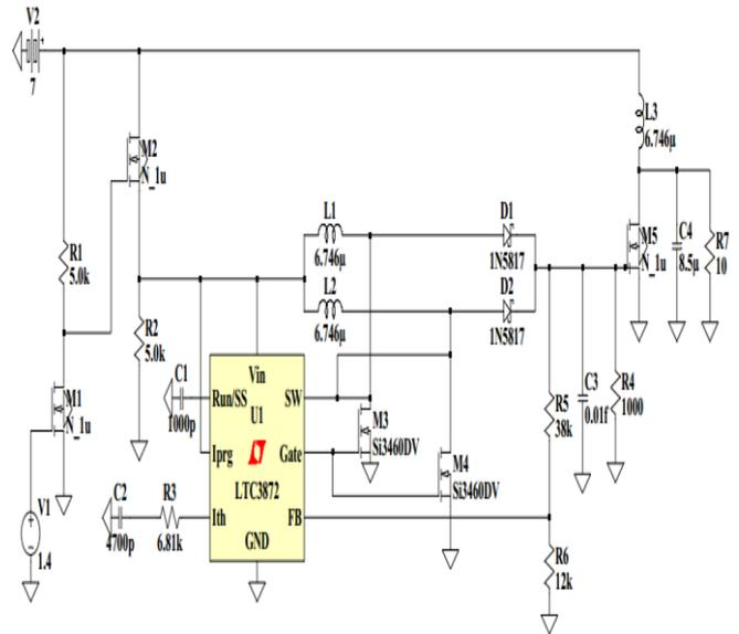
Fig. 6- Interleaved Boost Converter using LTC3872
