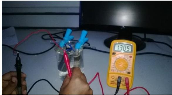
Fig. 7- Microbial Fuel Cell using sea water
