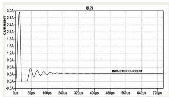
Fig. 11- Inductor current ripple of IBC
