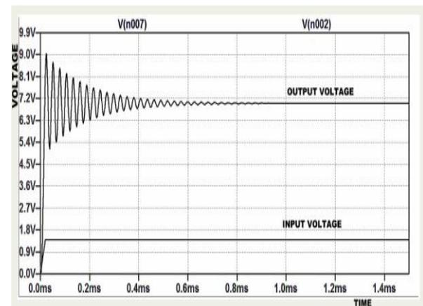
Fig. 19- Input and Output voltage of Boost Converter using LTC3872
