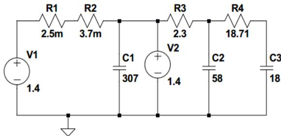
Fig. 4- Supercapacitor Model
