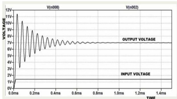
Fig. 16- Input and Output voltage of IBC using LTC3872
