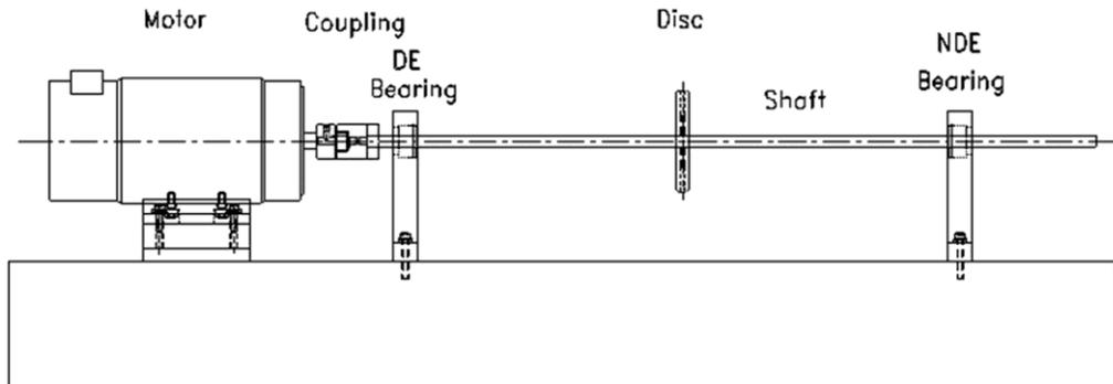
Fig. 1—Rotor-coupling-bearing test rig
