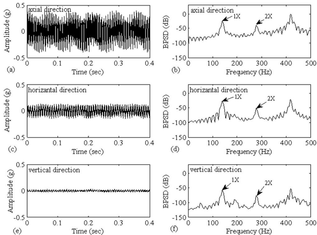
Fig. 2—The original vibration signals and Bartlett power spectral density of angular misalignment at 8400 rpm
