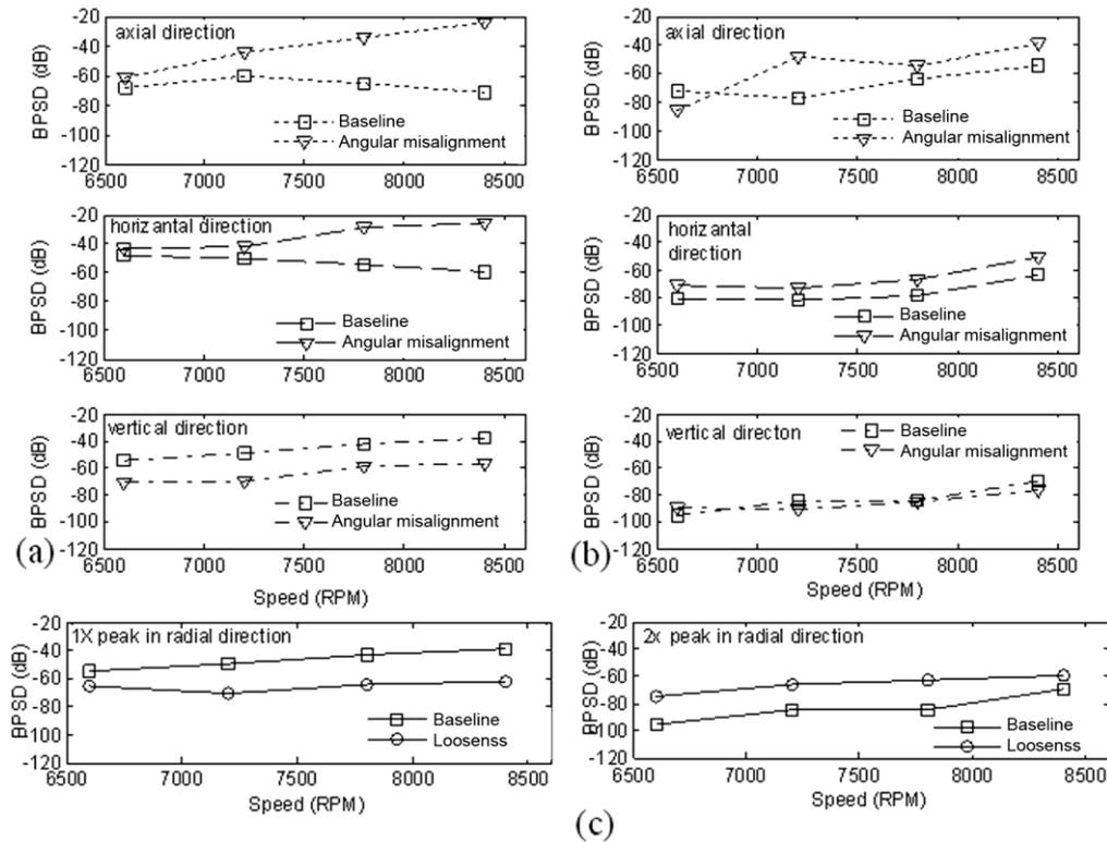
Fig. 3—Bartlett Power Spectral Density: (a) angular misalignment at 1X peak (b) angular misalignment at 2X peak and (c) Looseness at 1X peak and 2X peak
