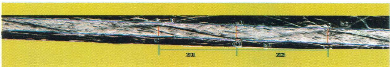
Fig. 2 – Tracer fibre measurement
