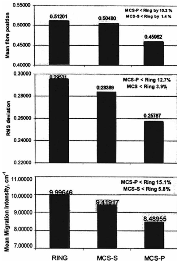
Fig. 3 – Mean fibre position ( $\bar{y}$ ), RMS deviation ( $D$ ) and mean migration intensity ( $I$ ) of 40s Ne yarn
