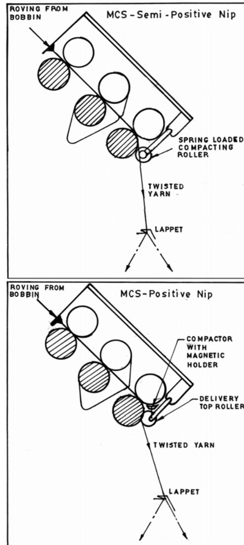
Fig. 1 – Schematic diagram of mechanical compacting system—semi-positive nip and positive nip
