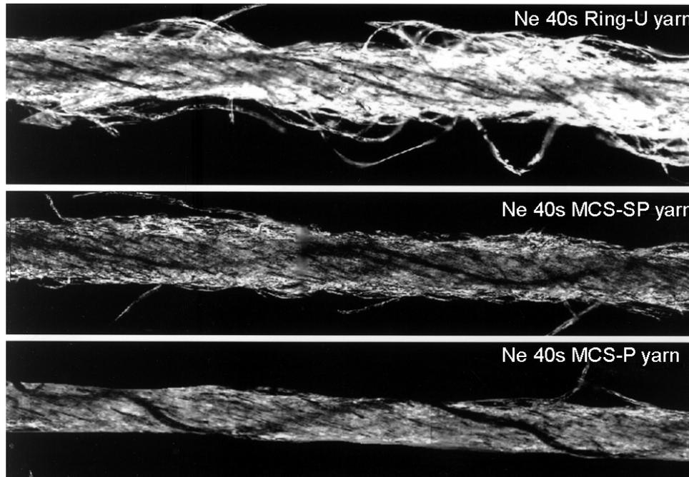
Fig. 5 – Ring, MCS-S and MCS-P yarns with tracer fibre
