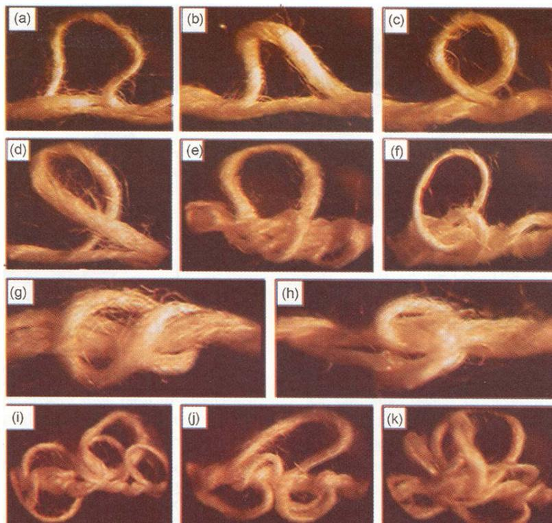
Fig. 3 — Microscopic pictures of effects in fancy yarns [(a), (b) – opened loop; (c), (d) – closed loop; (e), (f) – loop-knot; (g), (h) – plain knot; and (i), (j), (k) – knot made from various loops]
