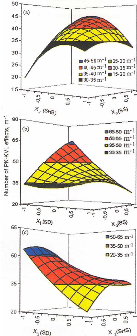
Fig. 4 — Dependence of number of effects of plain knot - knot made of various loops per unit length of fancy yarn on the (a) rotational speed of hollow spindle  $X_2$  (SHS) and the speed of supply of effect component  $X_3$  (SS); (b) delivery speed of fancy yarn  $X_1$  (SD) and the speed of supply of effect component  $X_3$  (SS); and (c) delivery speed of fancy yarn  $X_1$  (SD) and the rotational speed of hollow spindle  $X_2$  (SHS)
