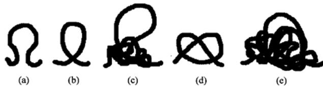
Fig. 2 — Various kinds of fancy effects [(a) opened loop, (b) closed loop, (c) loop-knot, (d) plain knot, and (e) knot made from various loops]
