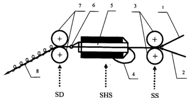
Fig. 1 — Principle of formation of effect intermediate product and fancy yarn using hollow spindle [1 – core component, 2 – effect component, 3 – supply rollers, 4 – binder component, 5 – hollow spindle with binder component, 6 – separator-regulator, 7 – delivery rollers, and 8 – fancy yarn]
