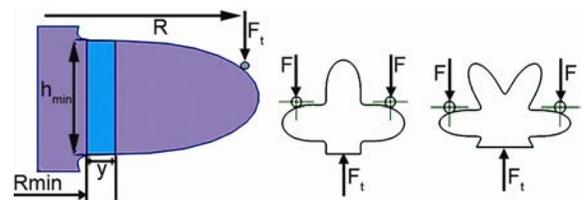
Fig. 4—Schematic view of loads on gears for fatigue test (a) detailed view of loading, (b) 4 teeth gear loading and (c) 6 teeth gear loading
