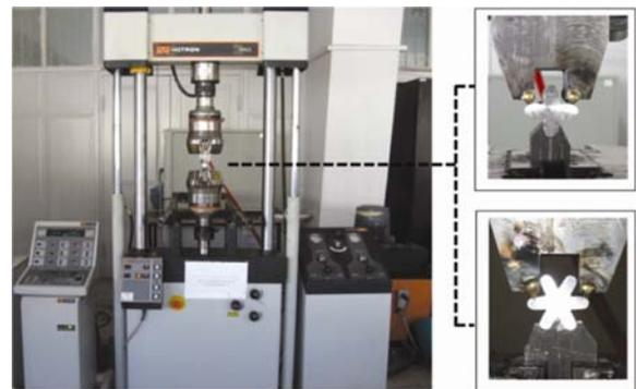
Fig. 3—Experimental setup of fatigue tests
