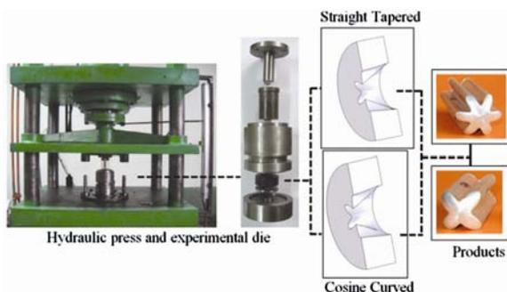
Fig. 2—Experimental die setup and extrusion products
