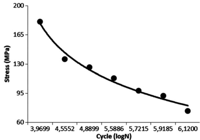
Fig. 6—Fatigue stress-cycle curve of 4 teeth cosine profile for 15 mm die land length
