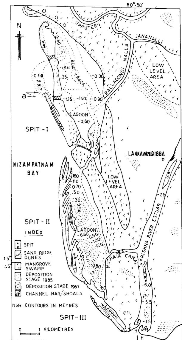
Fig. 3—Recent stage of barrier system development [based on present studies and surveys]
