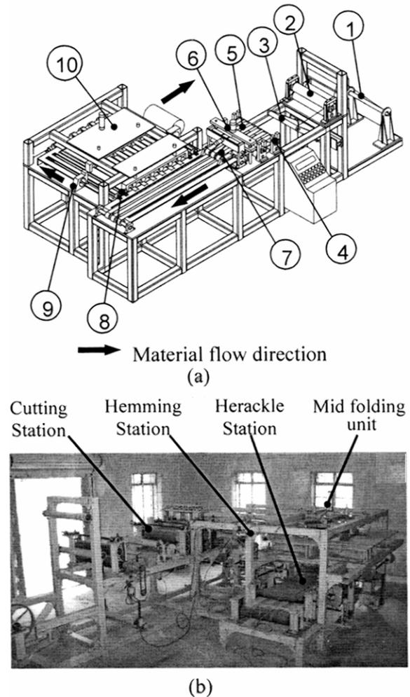
Fig. 1—(a) Schematic view and (b) perspective view of automatic jute bag making machine [1-mandrel, 2-feed roller assembly, 3-guide roller assembly, 4-dancing roller assembly, 5-conveyor assembly I, 6-shearing assembly, 7-gripper assembly I, 8-gripper assembly II, 9-stitching machines and 10-mid-folding unit]
