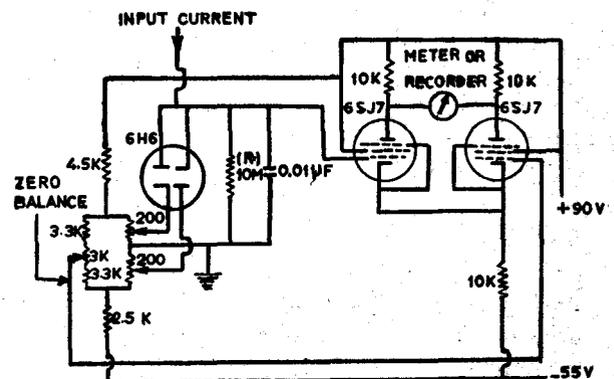
Fig. 1—Circuit diagram of bipolar logarithmic amplifier
