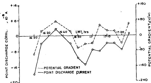
Fig. 3—Hourly variation of point discharge current and potential gradient during a typical disturbed weather day (11 May 1971)
