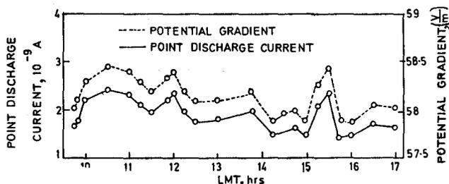
Fig. 2—Hourly variations of point discharge current and potential gradient during a typical fair weather day (20 Feb. 1971)
