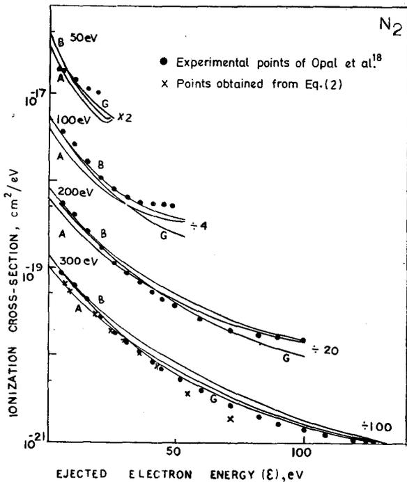
Fig. 2—Plots of cross-section  $Q(E, \epsilon)$  for electron impact ionization of  $N_2$  molecules for different values of  $E$  between 50 and 300 eV [Curve: B, obtained from Eq. (7) with original  $\partial f/\partial W$  values of Silvermann and Lessetre<sup>28</sup>; A, obtained from Eq. (7) with corrected  $\partial f/\partial W$  values of Silvermann and Lessetre<sup>28</sup>]
