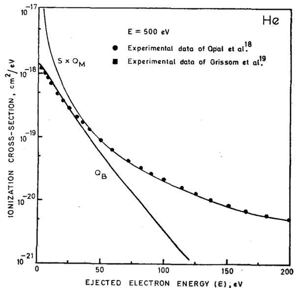
Fig. 1—Plots of cross-section  $Q(E, \epsilon)$  for He at  $E=500$  eV. [ $Q_B$  is obtained from Eq. (3) and  $SQ_M$  from Eq. (5) with  $S=2$  ● and ▲ are the experimental data of Opal *et al.*<sup>18</sup> and Gissom *et al.*<sup>19</sup>, respectively.]
