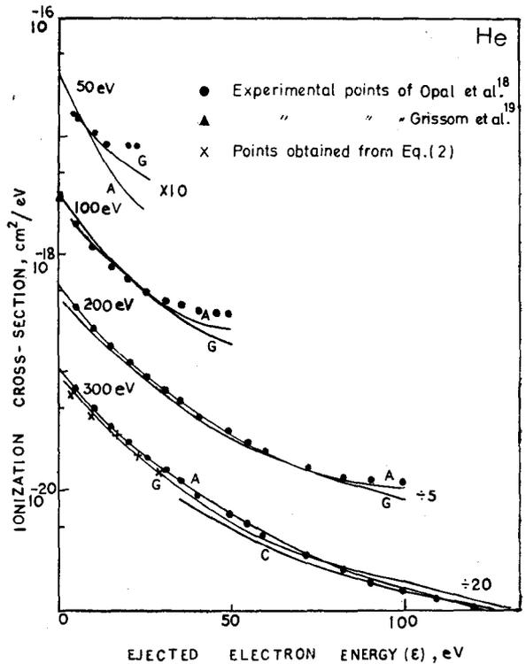
Fig. 4—Cross-section  $Q(E, \epsilon)$  for electron impact ionization of He atoms for the values of  $E$  lying in the range 50-300 eV [Curve: A, obtained from Eq. (7); G, from Eq. (13); C, from Eq. (2)]
