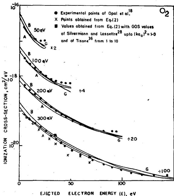
Fig. 6—Cross-section  $Q(E, \epsilon)$  for electron impact ionization of O<sub>2</sub> molecules for the values of  $E$  lying in the range 50-300 eV [See caption of Fig. 2 for other details]
