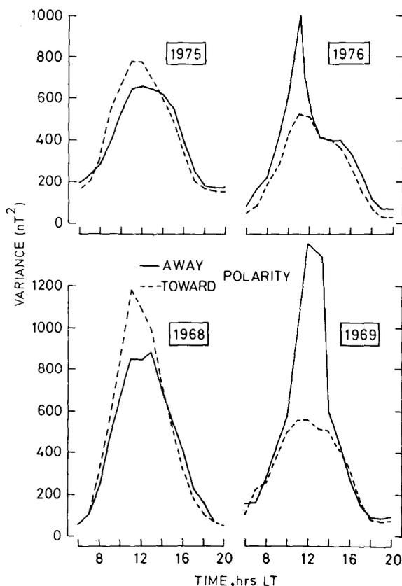
Fig. 2—Variability of equatorial electrojet strength as a function of 75° EMT for four years (The variances are computed for two categories based on polarity of the interplanetary magnetic field).
