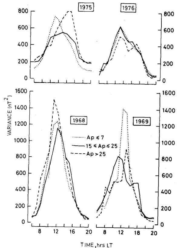
Fig. 1—Variability of equatorial electrojet strength (taken as the difference in  $H$  field at Trivandrum and Alibag) as a function of 75° EMT for solar maximum and minimum years (The variances are computed for three categories of magnetic activity).
