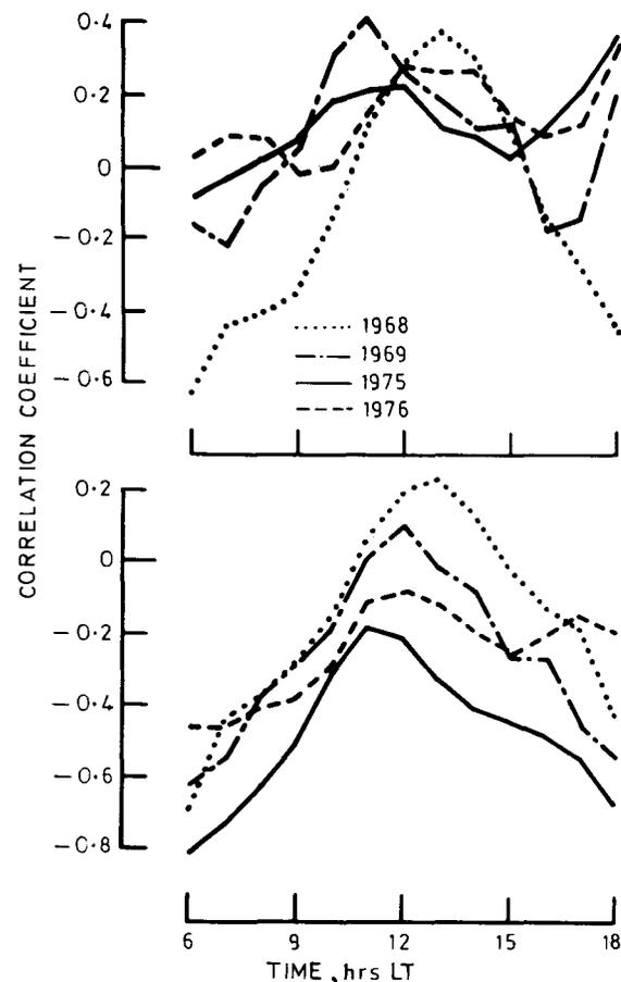
Fig. 6—Local time dependence of the correlation between ionospheric part of the daily variation at low latitude [ $SDI(LL)$ ] and (i)  $SDI(EQ)$  (top) and (ii) Electrojet strength (bottom) for four years [It may be noted that the correlation coefficient is computed using 365 (366) values for each year.]
