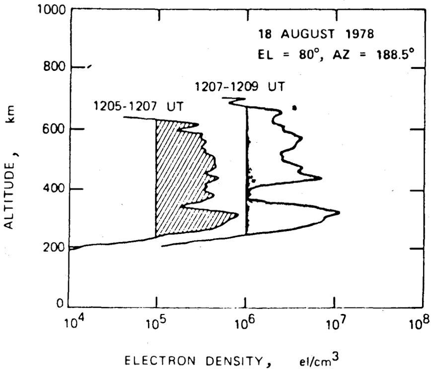
Fig.2 — Height profiles of electron density at Kwajalein (4.3°N dip latitude) as measured with the ALTAIR Incoherent Scatter radar during spread F conditions (Tsunoda 1980).
