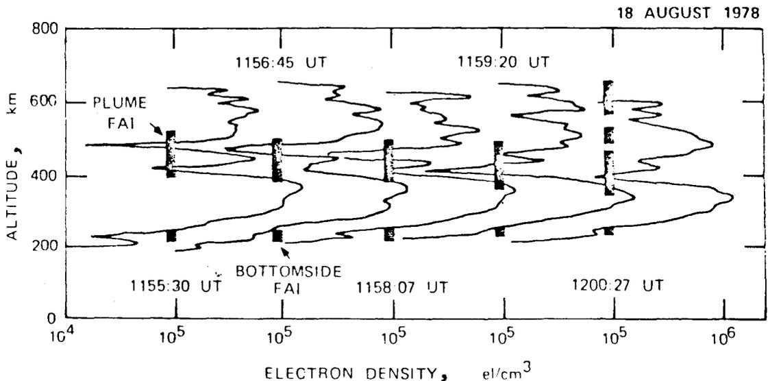
Fig.4— Height profiles of electron density exhibiting large depletions in narrow height regions; dark vertical bands represent the regions from which intense backscatter signals at 155 MHz (i.e. from 1-m size irregularities) were observed at Kwajalein (Tsunoda 1980).
