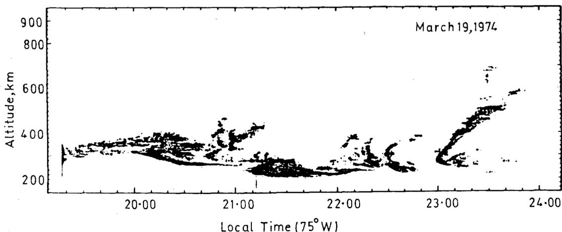
Fig.1— Time - height cross-section of backscatter signals from 3-m size ionization irregularities in F-region at Jicamarca, Peru. The upward and downward movements of backscattering regions and their total disappearance for a brief period around 2255 hrs. are to be noted (Woodman and La Hoz 1976).
