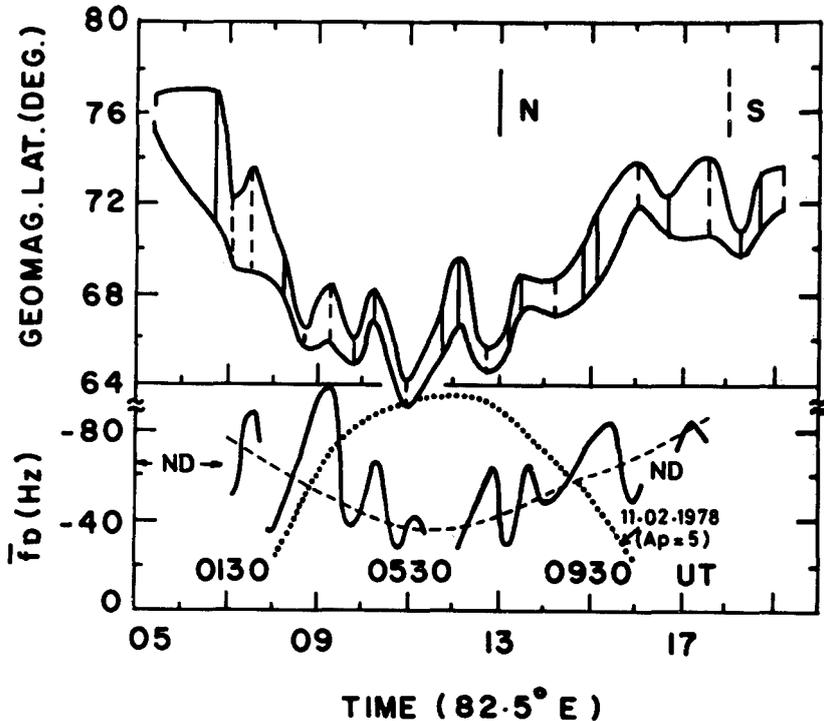
Fig.8— In-phase variations of the mean Doppler frequency  $\bar{f}_D$  of backscatter radar signals from electrojet at Thumba and the latitude of the polar cusp.  $\bar{f}_D$  is proportional to the electric field in the electrojet (Somayajulu et al 1985).
