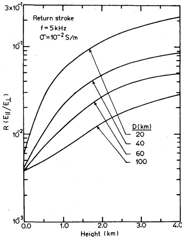
Fig. 4—Variation of  $R$  with height for a return stroke
