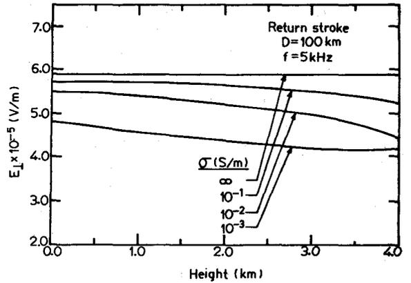
Fig. 2a—Variation of vertical electric field,  $E_{\perp}$ , with height for different ground conductivities for a return stroke
