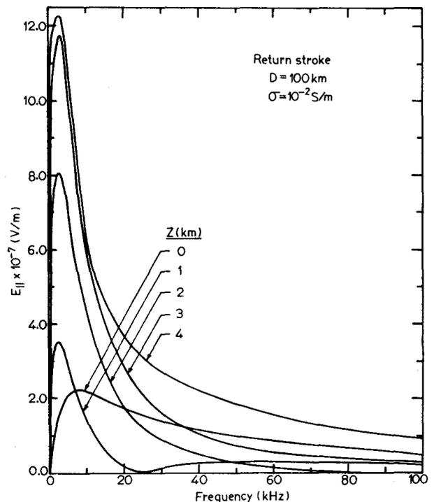
Fig. 3b—Variation of  $E_{\parallel}$  with frequency for different  $Z$  ( $\sigma = 10^{-2}$  S/m)
