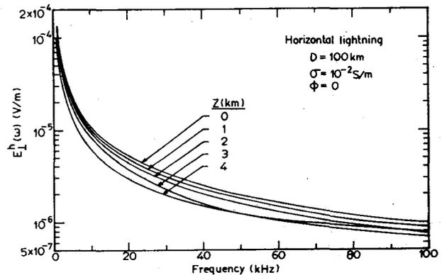
Fig. 5a—Variation of  $E_{\perp}^h(\omega)$  with frequency for different  $Z$  ( $\sigma = 10^{-2}$  S/m and  $\phi=0$  for horizontal lightning)
