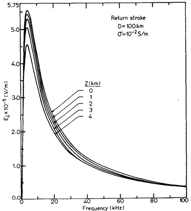
Fig. 3a—Variation of  $E_{\perp}$  with frequency of radiation for different heights of point of observation  $Z$  ( $\sigma = 10^{-2}$  S/m)
