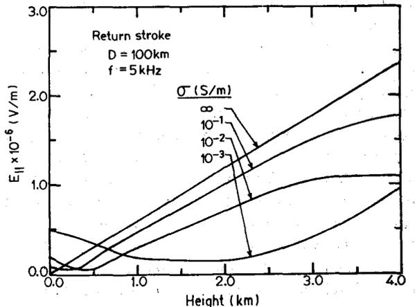
Fig. 2b—Variation of horizontal electric field,  $E_{\parallel}$ , with height for different ground conductivities for a return stroke.
