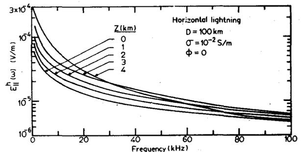
Fig. 5b—Variation of  $E_{\parallel}^h(\omega)$  with frequency for different  $Z$  ( $\sigma = 10^{-2}$  S/m and  $\phi=0$  for horizontal lightning)
