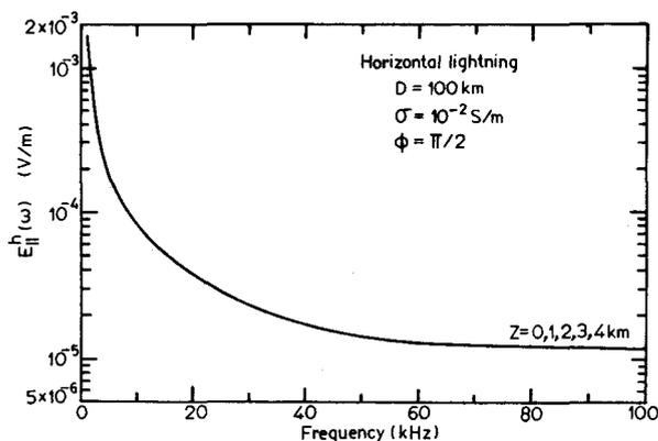
Fig. 6—Variation of  $E_{||}^h(\omega)$  with frequency for  $\sigma = 10^{-2}$  S/m and  $\phi = \pi/2$  for a horizontal lightning
