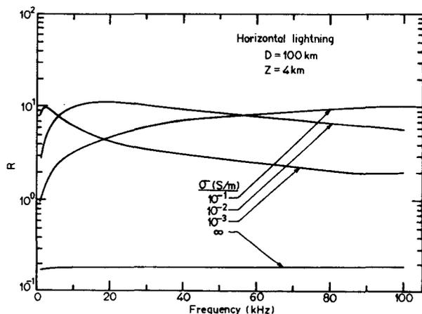
Fig. 7—Variation of  $R$  with frequency for horizontal lightning
