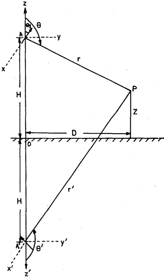
Fig. 1—Geometry of an arbitrarily oriented lightning channel (P is the point of observation in space)
