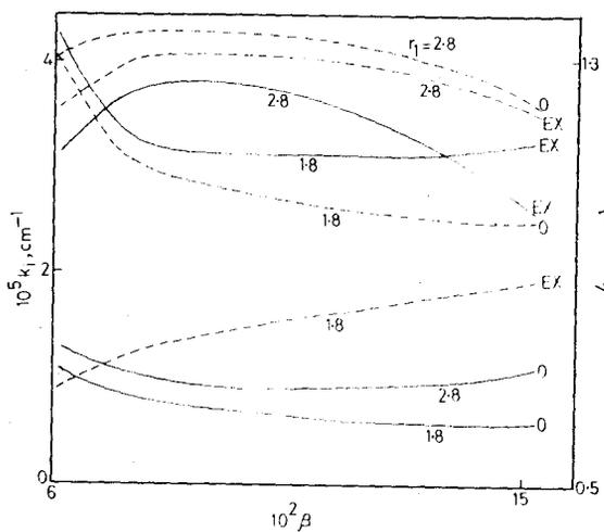
Fig. 2—Plot of  $k_i$  (solid line) and wave number  $k_r$  (broken line) versus  $\beta$  for  $L=3$ ,  $\theta=60^\circ$ ,  $r_1=1.8$  and  $2.8$
