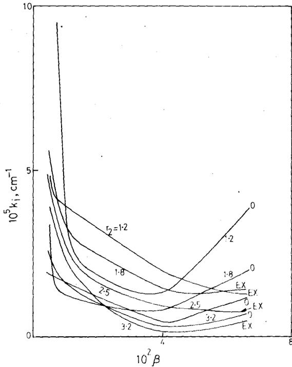
Fig. 1—Plots of growth rate  $k_i$  versus  $\beta$  for ordinary (O) and extraordinary (EX) mode for  $L=2$ ,  $\theta=60^\circ$ ,  $r_2=1.2, 1.8, 2.5$  and  $3.2$
