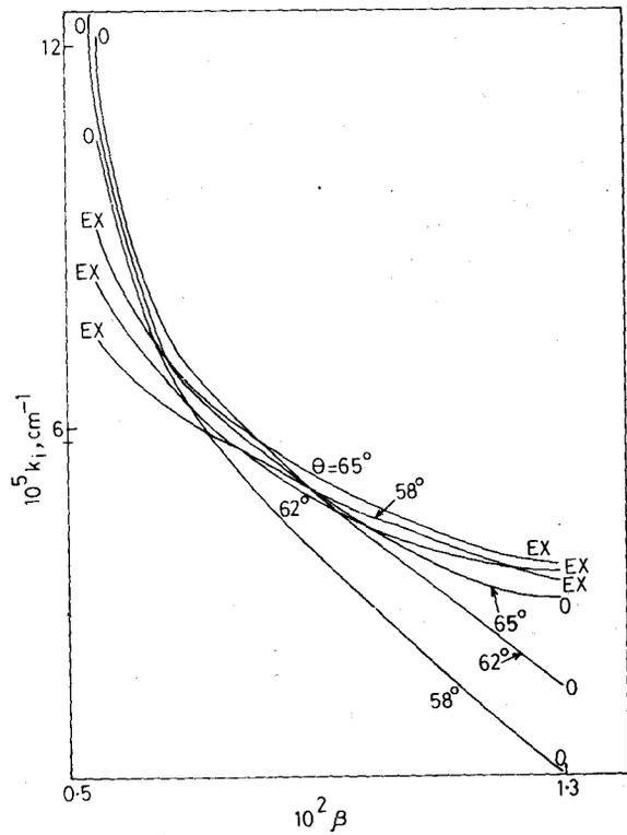
Fig. 3—Plot of  $k_i$  versus  $\beta$  for  $L=2$ ,  $r_1=2.2$ ,  $\theta=58^\circ, 62^\circ$  and  $65^\circ$
