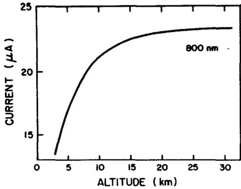
Fig. 4—Photometer current corresponding to 800 nm
