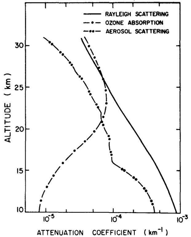
Fig. 5—Altitude variations of the computed attenuation coefficients for 800 nm corresponding to Rayleigh scattering, ozone absorption and aerosol scattering
