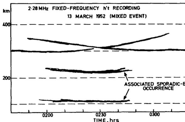
Fig. 1 - Example of a mixed spread-F event recorded at fixed frequency (after McNicol *et al.*<sup>2</sup>)
