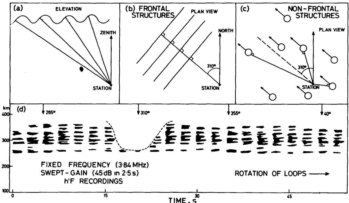
Fig. 4 - (a) Elevation view and (b) plan view of suggested frontal structures; (c) plan view of non-frontal structures; and (d) simulated rotating-loops recording showing azimuths-of-arrival of around 310° (after Bowman<sup>3</sup>)
