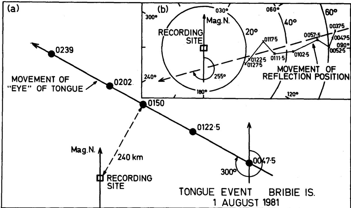
Fig. 7—For a “tongue” event on 1 Aug. 1981: (a) general movement of the large-scale structure, and (b) movement of the reflecting point as it changes position on the large-scale structure
