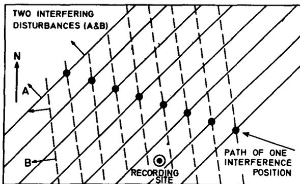
Fig. 8 – Diagrammatic illustration of two interfering wave-trains travelling in different directions
