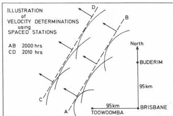
Fig. 3 – Diagram illustrating method used by McNicol *et al.*<sup>2</sup> to calculate speeds and directions of travel of spread-F TIDs
