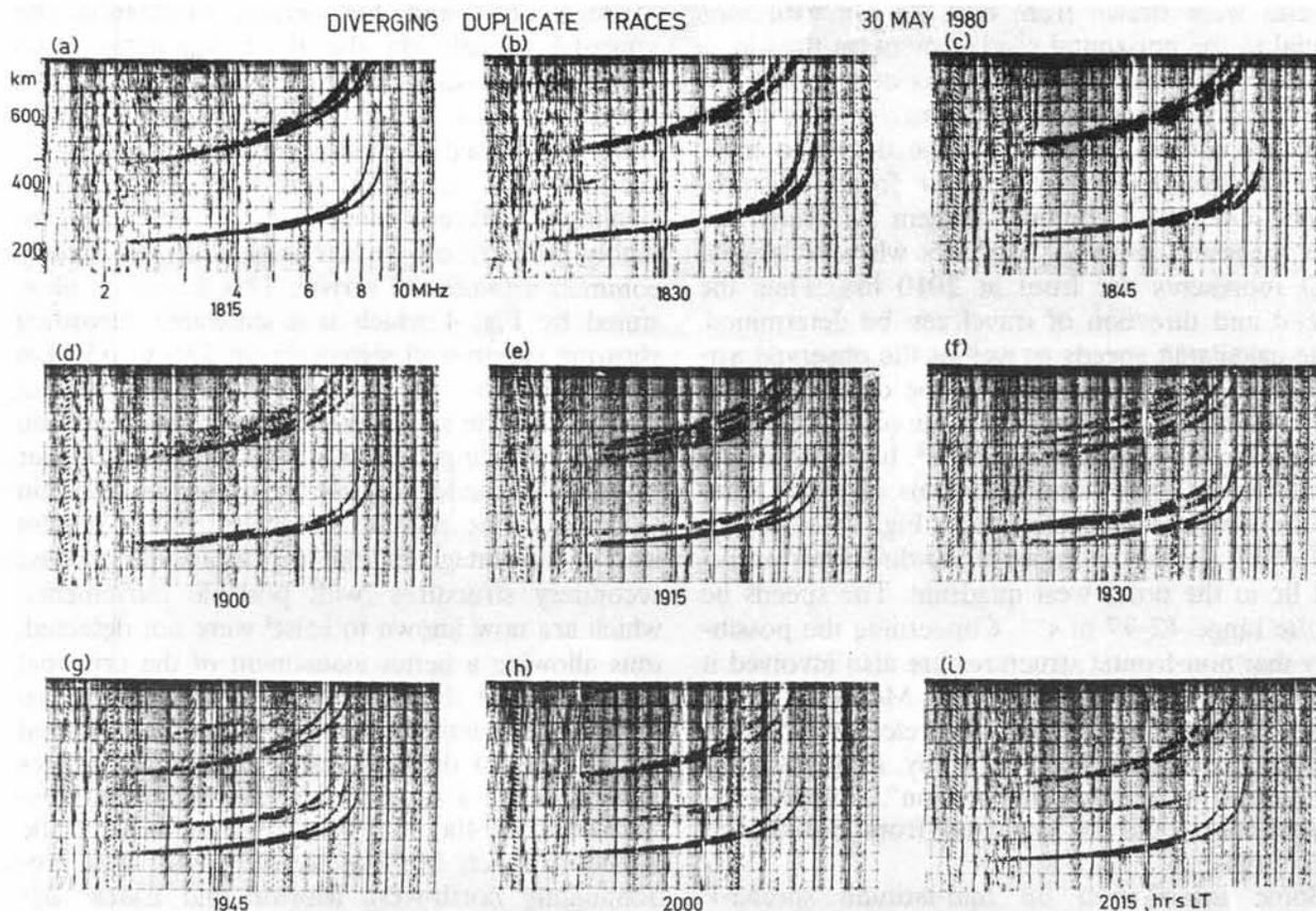
Fig. 2 – Example of diverging duplicate spread-F traces as observed on ionograms recorded at Brisbane on 30 May 1980
