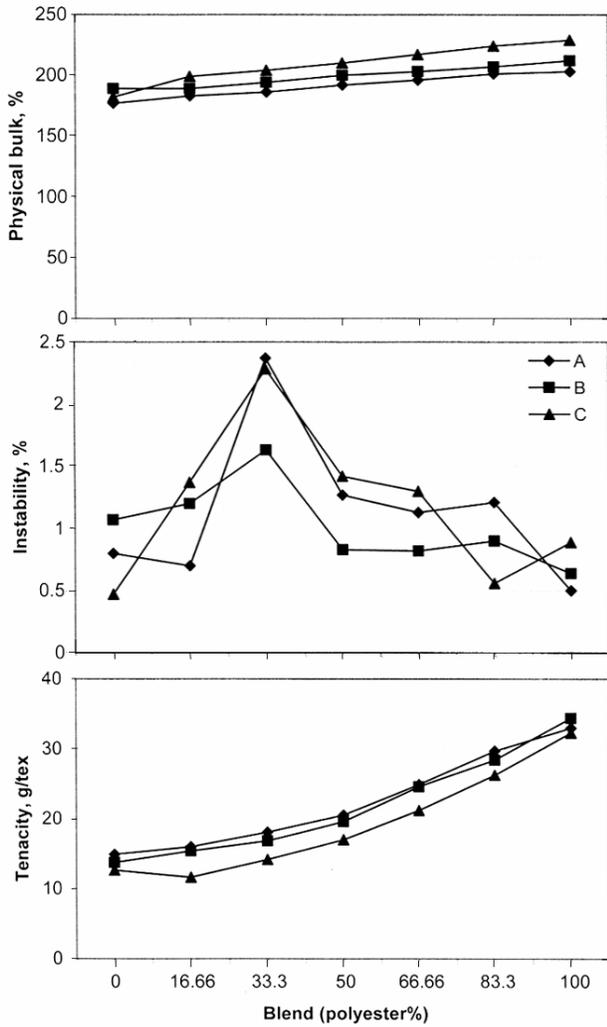
Fig. 1—Effect of blend proportion on yarn physical bulk, instability and tenacity at 400m/min texturing speed [(A) 14.7% overfeed, 7 bar air pressure, (B) 24% overfeed, 8.5 bar air pressure, and (C) 33.3% overfeed, 10 bar air pressure]
