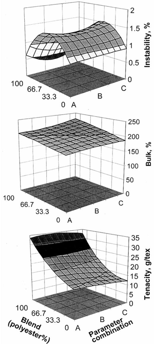
Fig. 2—Interaction effect of blend percentage and process parameters on yarn Instability, physical bulk and tenacity at constant texturing speed of 400 m/min
