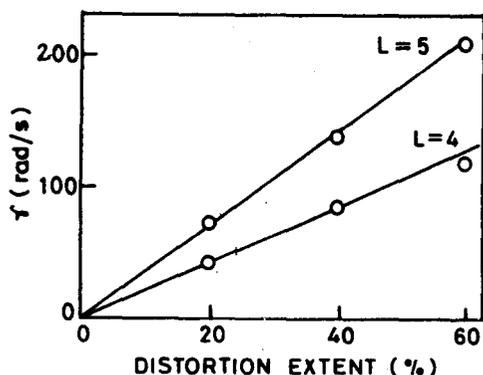
Fig. 2—Variation of per cent increment in temporal growth rate ( $\gamma$ ) with distortion extents at  $L=4$  and  $L=5$ .
