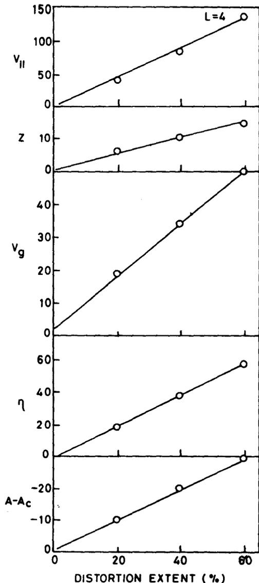
Fig. 1—Variations of per cent changes in  $V_{||}$ ,  $Z$ ,  $V_g$ ,  $\eta$  and  $(A-A_c)$  with distortion extents at  $L=4$ .
