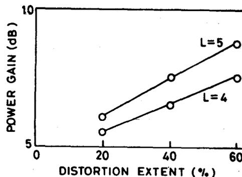
Fig. 3—Variation of per cent increment in power gain with distortion extents at  $L=4$  and  $L=5$ .
