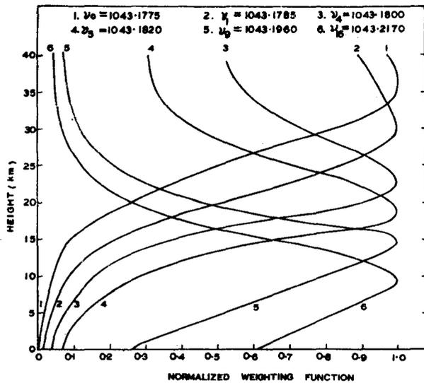
Fig. 4—Normalized absorption coefficients for different channels at the line centre and in the wing of the line as a function of altitude.
