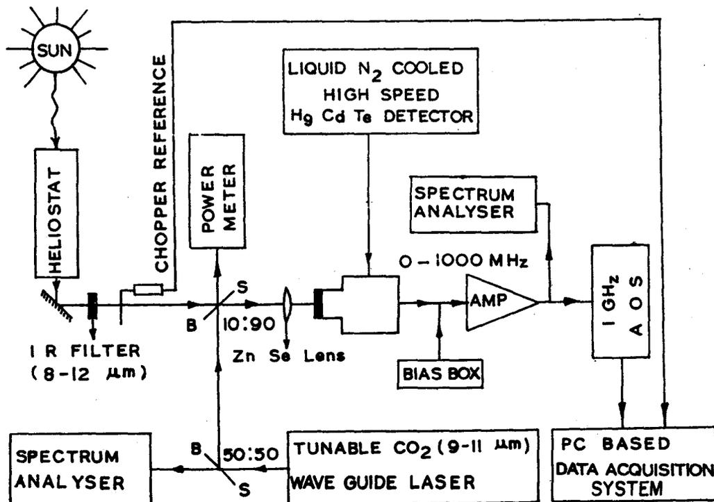
Fig. 1—Block diagram of laser heterodyne system of NPL, New Delhi.
