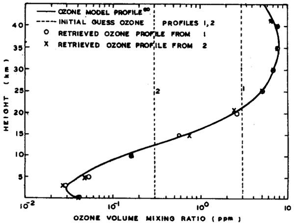
Fig. 6—Model and retrieved ozone height profiles obtained using inversion technique (normal case).
