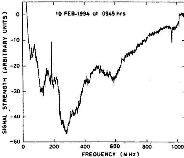
Fig. 3—Line spectra of ozone observed at Maitri, Antarctica, on 10 Feb. 1994.
