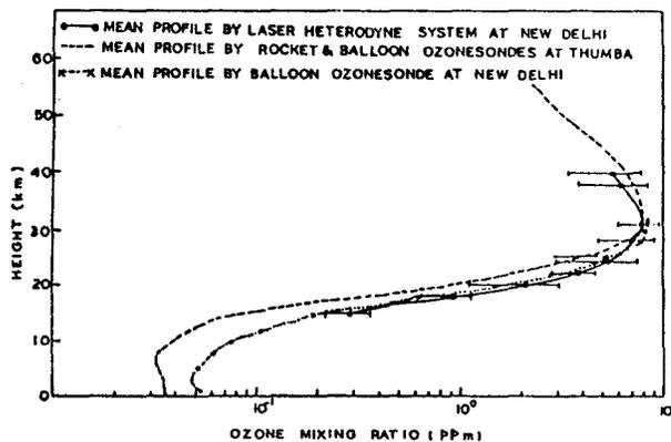
Fig. 9—Comparison of mean ozone vertical profiles obtained by (a) laser heterodyne system at NPL, New Delhi, (b) balloon ozonesonde at Aya Nagar, New Delhi, and (c) rocket and balloon ozonesondes at Thumba.
