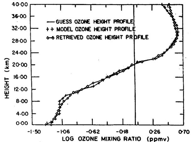
Fig. 7—Antarctica model profile<sup>61</sup> and retrieved ozone profile obtained using inversion technique (ozone hole case).
