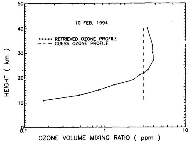
Fig. 10—Ozone profile obtained by laser heterodyne system on 10 Feb. 1994 over Maitri, Antarctica.
