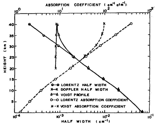
Fig. 5—Line half-widths and absorption coefficients for ozone obtained using Lorentz, Doppler and Voigt profiles.
