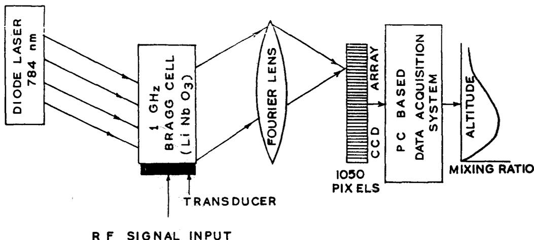
Fig. 2—Block diagram of acousto-optic spectrometer.
