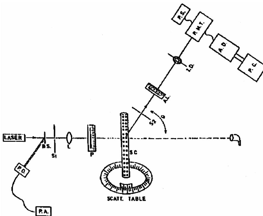
Fig. 1—Homemade laser light scattering spectrometer. [B.S., Beam splitter; P.D., photo diode; P.A., pico ammeter; S<sub>1</sub>, S<sub>2</sub>, slits; L, lens; P, polarizer; S.C., scattering cell; A.L., analyzer; I.D., iris diaphragm; P.M.T., photo multiplier tube; A.D., amplifier discriminator; P.C., photon counter; P.S., power supply]
