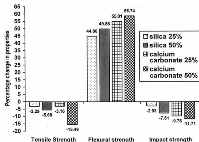
Fig. 1 — Percentage difference in properties in comparison to without filler sample
