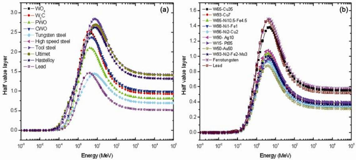
Fig. 2—The variation of half value layer of tungsten compounds, alloys and lead in the photon energy range 1 keV to 100 GeV
