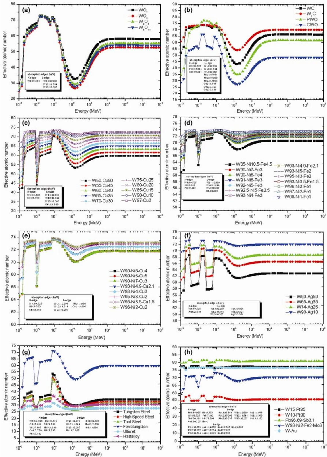
Fig. 1—The variation effective atomic numbers of tungsten compounds, alloys and lead in the photon energy ranging 1 keV to 100 GeV
