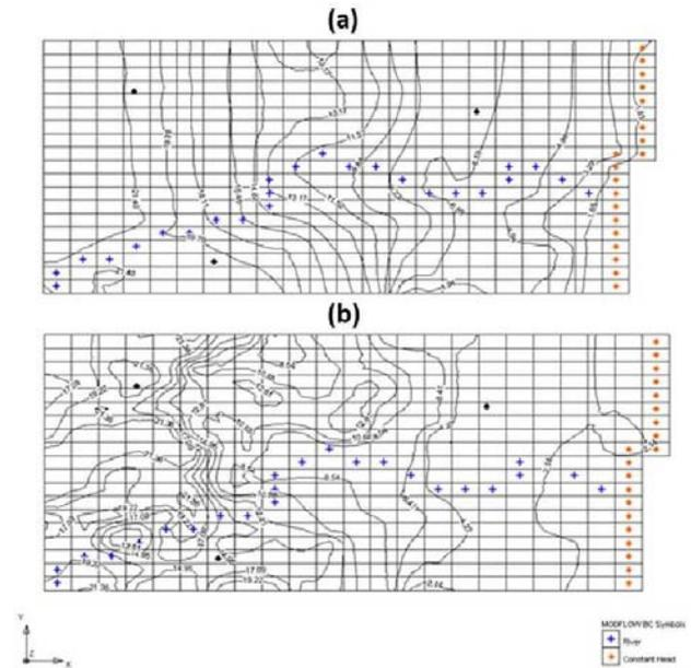
Fig. 2—Simulated groundwater level (masl) in Chennai city (a) with present level of rainfall recharge and (b) with anticipated increase in recharge with rainwater harvesting structures (+ - Adyar River, \* - Bay of Bengal)
