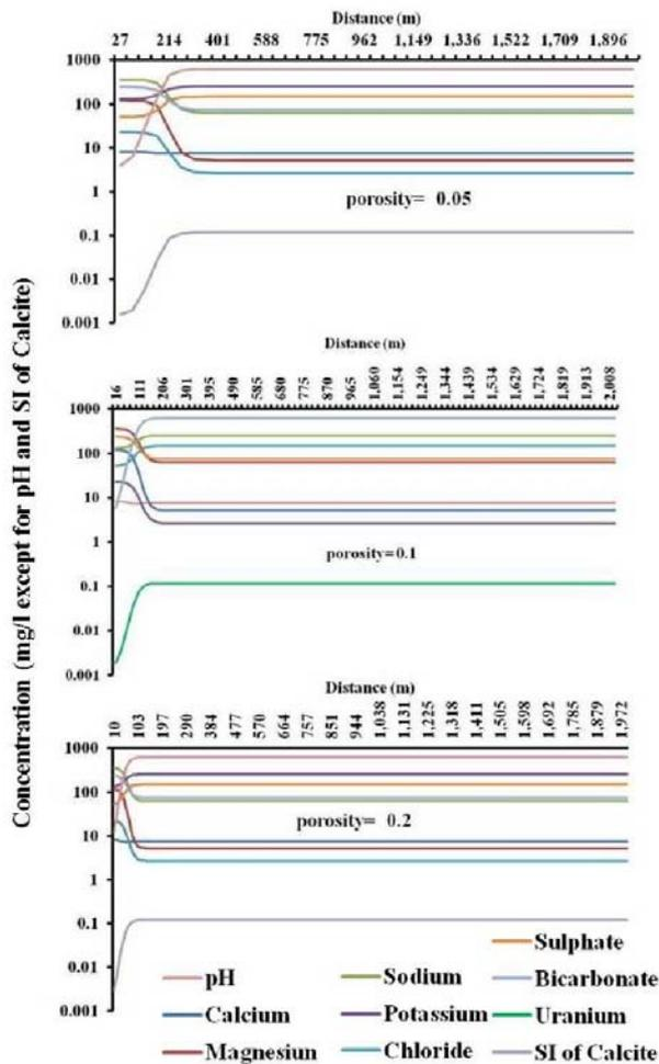
Fig. 4—Variation in the movement of ions at the end of 100 years at different porosity from a uranium tailings pond
